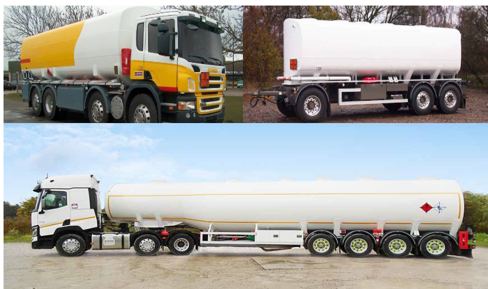
Figure 23: a) Tank, b) trailer, and c) tank trailer (semi-trailer)
