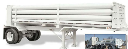
Figure 29: Trailer and storage is same vessel.
