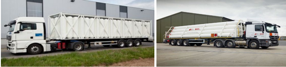
Figure 25: Hydrogen tube trailer types
