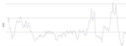
Figure 38 : The load varies throughout the week. The measurement accounts for both operating and idle periods, as well as the complete installation including the air dryer
