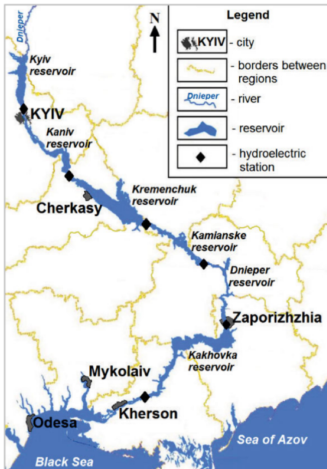
Figure 35: Dnieper River dams and cascading system
