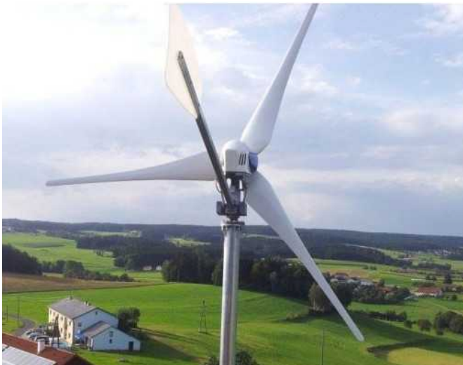
Figure 19: ANTARIS 2.5 kW household wind turbines
