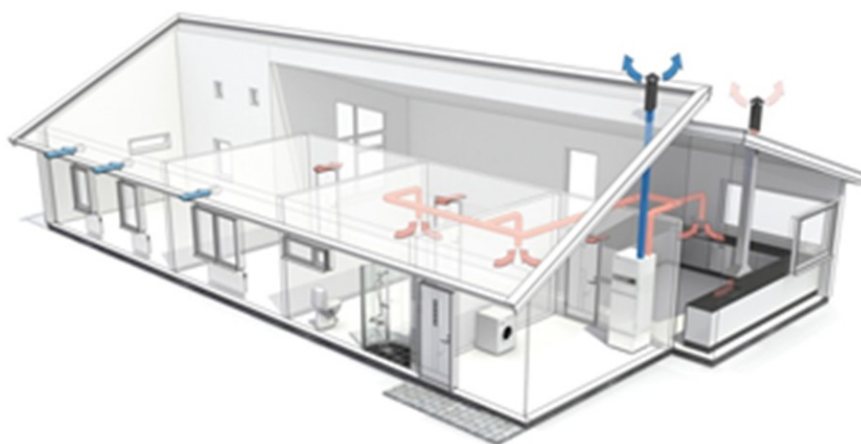
Figure 34 Illustration of a heating system based on a ventilation heat pump.
