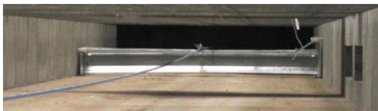
Figure 5. Mechanical scraper in manure channel under the slatted floor of a dairy barn. (Photo: Lind Jensens Maskinfabrik A/S).
