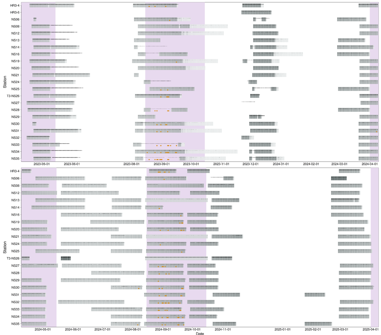
Figure 4.2. Deployment overview for the 22 bat PAM stations on buoys. Top: results from the first survey year (10. April, 2023, to 9. April, 2024). Bottom: results from the second survey year (10. April, 2024, to 9. April, 2025). Due to a mix-up during the deployment in winter, 2023, NS28 was deployed at the location of HR3_6. For this reason, the overview from the first year includes 23 stations. This was corrected during the following deployment. Orange points show nights where bats were recorded and are not scaled by the number of detections per night. Greyscale bars and black points are both indicators of recorder functionality. Grey bars are colour-scaled by the number of summary entries made by the recorder per night and fade into lighter shades recorders ran out of power and recorded only partially through the night. Black points indicate that a recorder was triggered during that night and made recordings, but those only included bats where black and orange points coincide on the same night. The black points are scaled by the number of trigger events (larger: more recordings triggered, smaller: fewer recordings triggered) and are present without grey bars for deployments where recorder summary files could not be recovered. The fact that recordings were still triggered indicates intact recorder functionality. Absence of black points means that no recording was triggered. Purple shading: expected migration periods based on literature.
