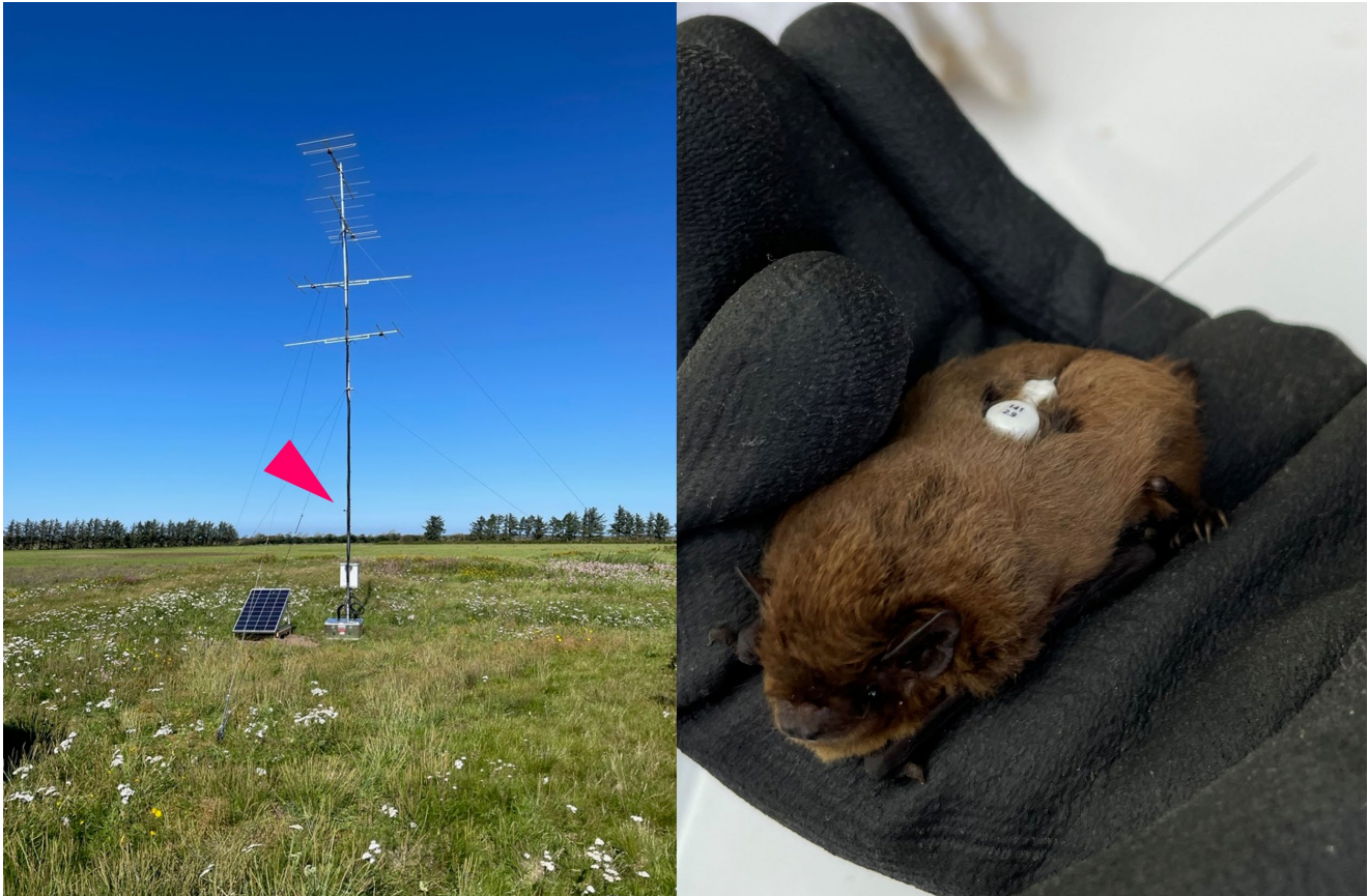
Figure 1.4. Photos from the onshore PAM and Motus components. Left: combined coastal PAM and Motus receiver station. The arrowhead indicates placement of the SM4BAT FS microphone. Right: Nathusius' pipistrelle ready for release with Motus radio-tag. Photo credits: L Haugaard and S Brinkløv/Aarhus University.
