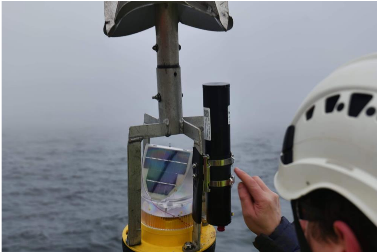
Figure 8 - PAM bat detector mounted on a buoy used for the marine mammal survey.
