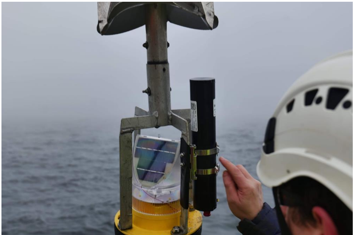
Figure 5 - PAM bat detector mounted on a buoy used for the C-POD station in the marine mammal survey.
