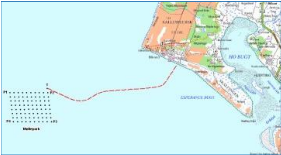
Figure 1. Location of the Wind Farm and the export cable which connects the substation to the onshore transmission grid.
