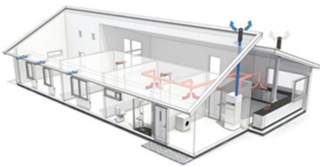
Figure 5 Illustration of a heating system based on a ventilation heat pump
