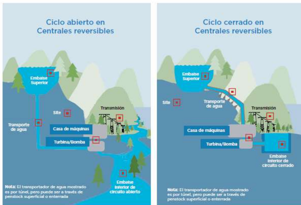
Figure 128. Main features of HPS installations for open cycle configurations (left) and closed cycle configurations (right) [1].
