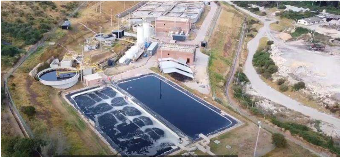
Figure 99. Leachate collection and treatment pond at Doña Juana Landfill [15].
