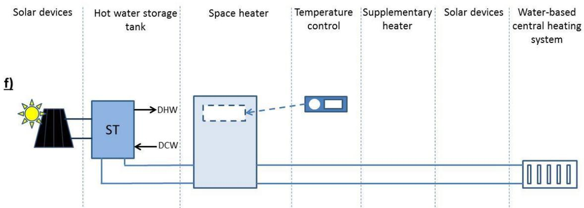
Figure 3 Example of package containing space heaters, where the solar devices are not part of the package
