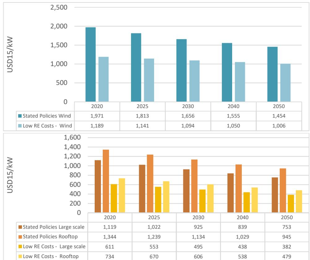
Figure 30: Investment cost assumptions in wind and solar PV projects in the Stated Policies and Low RE Costs scenarios, respectively (USD15/kW)
