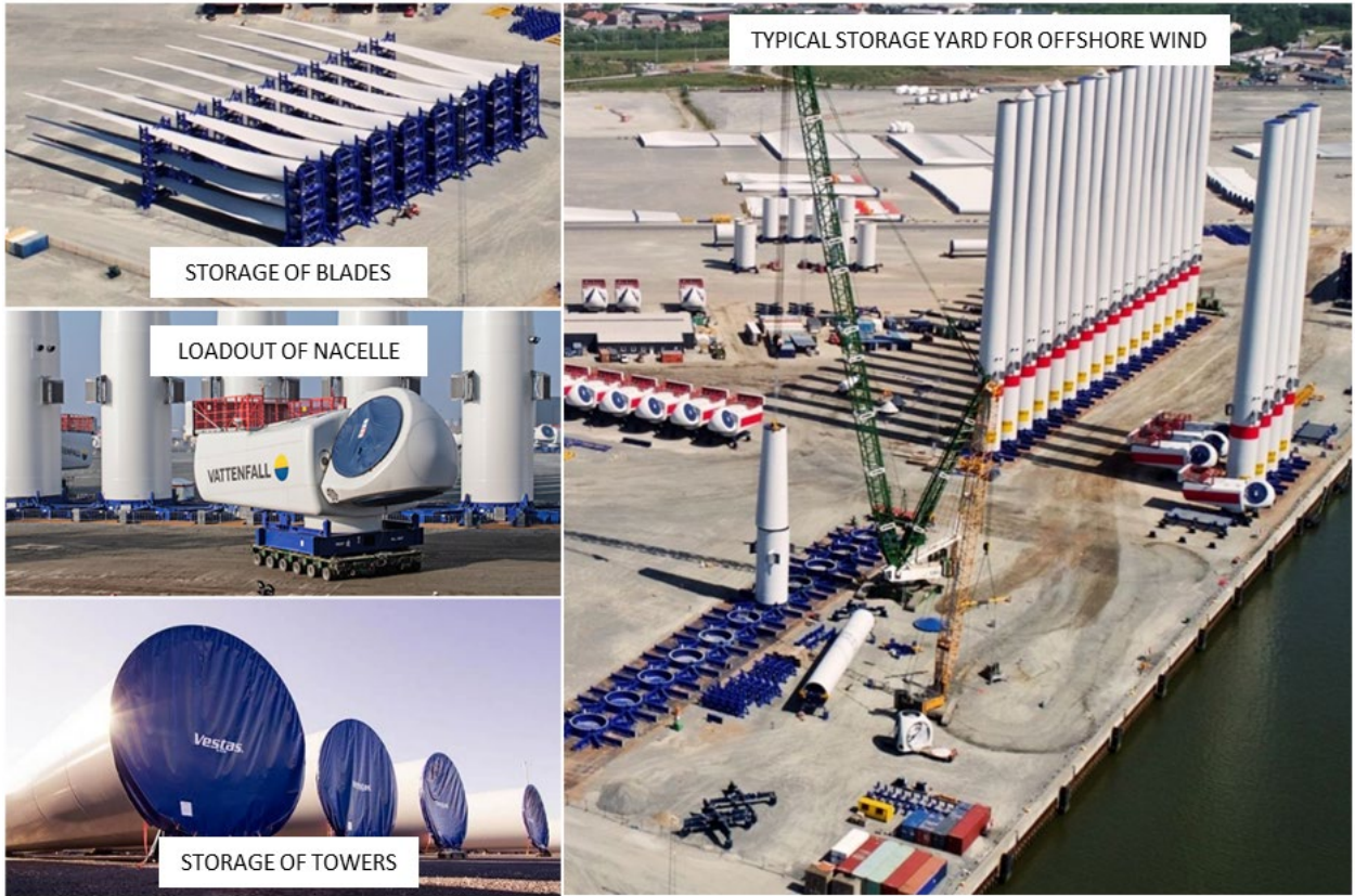
Figure 5-4: Blade, nacelle, tower storage operations
