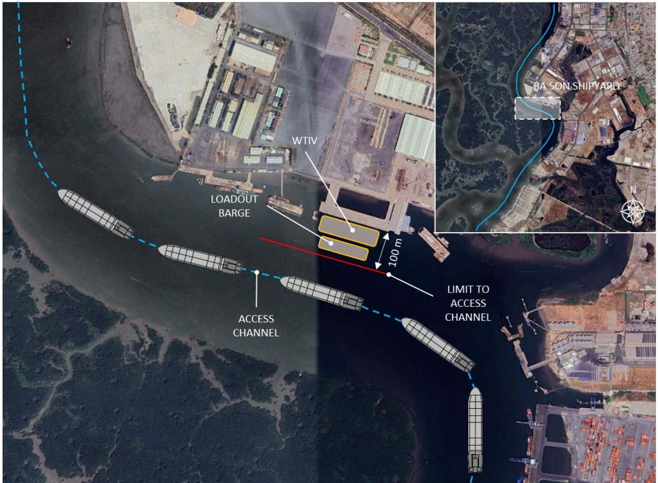
Figure 7-15: Access channel buffer zone
