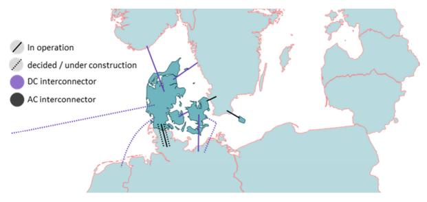
Figure 41 shows the existing and adopted Danish interconnectors included in PGSO-IP18, including the Great Belt Link. The link between Sweden and Bornholm has not been included in the power and gas sector outlook.
