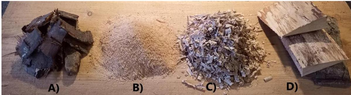
**Figure 4: Typical examples of industrial residues. A) Bark (Hog fuel), low quality, typically used for drying of wood pellets. B) Sawdust from sawmills, high quality clean wood, typically used for wood pellets. C) Planer shavings, from furniture production, high quality clean wood, typically used for wood pellets. D) Shells from sawmills, varying quality, typically used for wood chips or wood pellets.**
