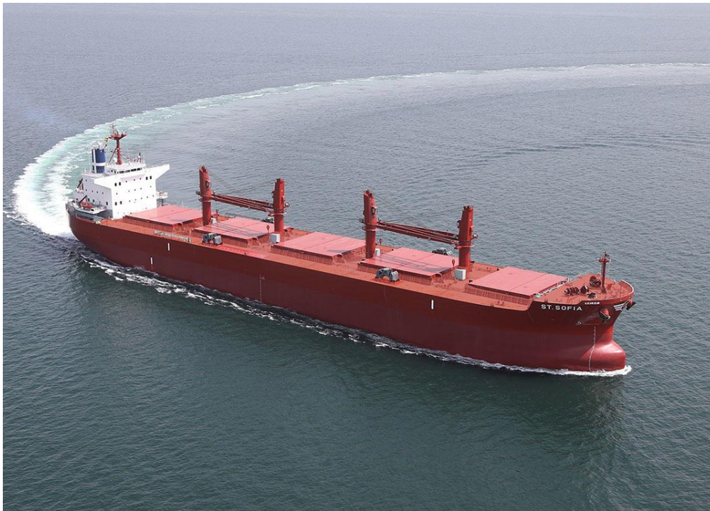
Figure 15 Bulk carrier 60,000 DWT (Copyright Mitsui E&S Shipbuilding)
