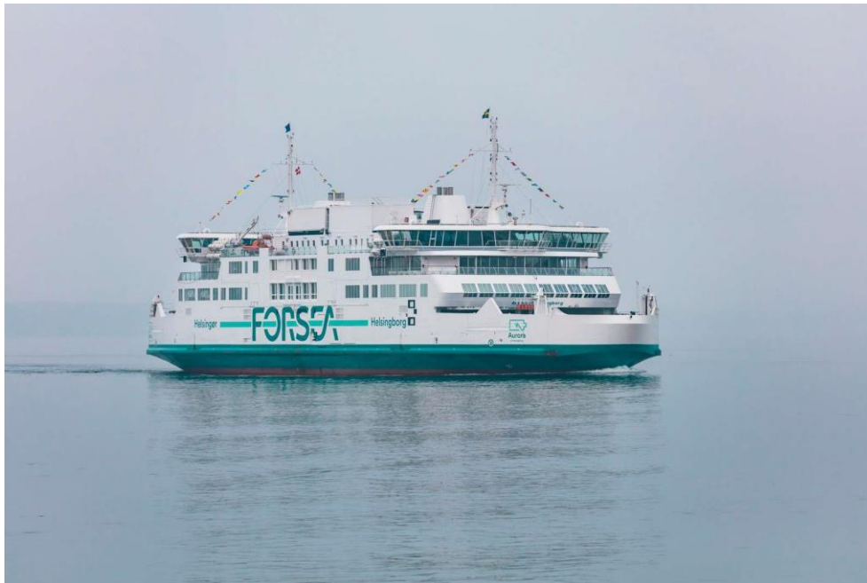
Figure 25 The battery-electric ferry Aurora operating the 2.5 nautical mile route between Elsinore, Denmark, and Helsingborg, Sweden (Courtesy of ForSea)
