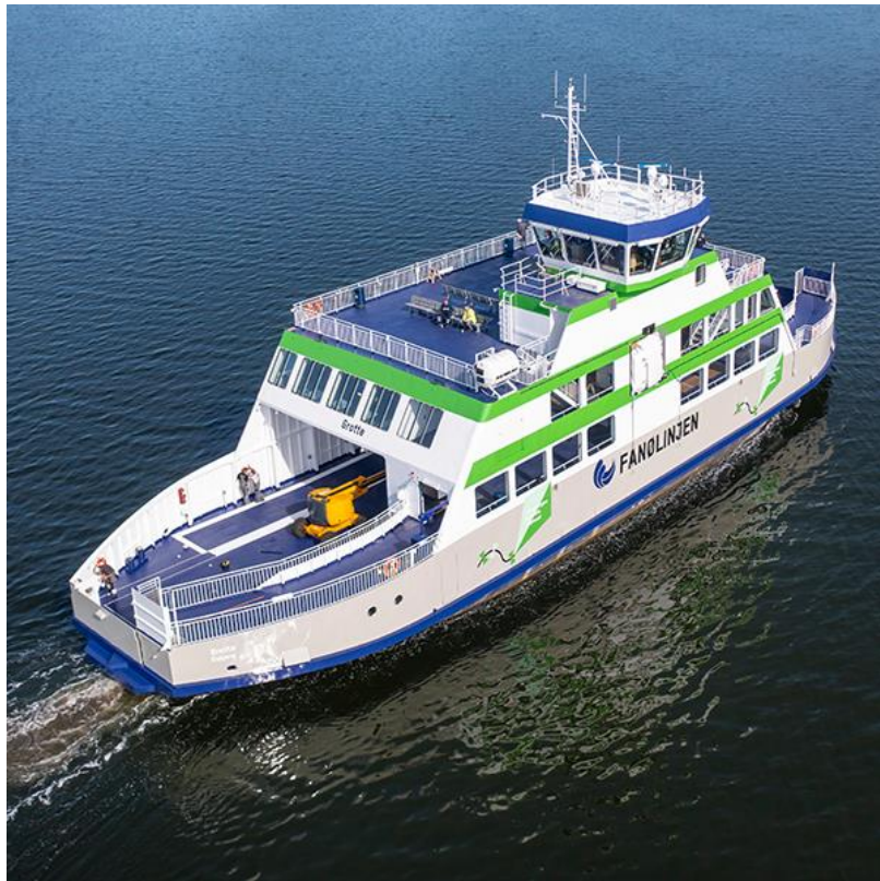
Figure 26 The battery electric ferry Grotte , operating the 1.35 nautical mile route between Fanø and Esbjerg (Courtesy Fanoelinjen)
