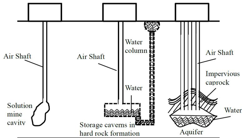
Figure 2: Various Geological Formations for Underground Storage [5]
