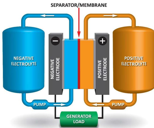
Figure 1: Schematic of flow battery [1].
