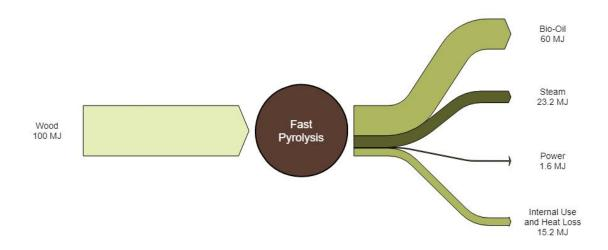
Figure 2 Fast Pyrolysis Oil Energy Balance
