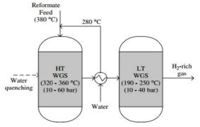
Figure 6: Typically shift configuration in an ammonia plant
