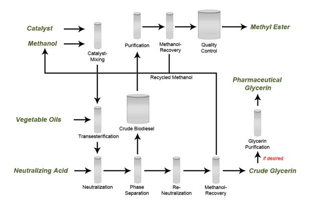
**Figure 1 Biodiesel Production Process**
