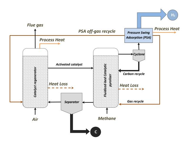
Figure 5. Fluidized Bed Catalytic-assisted Decomposition Diagram.
