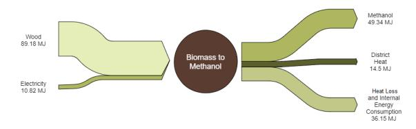
Figure 2 Bio Methanol Energy Balance
