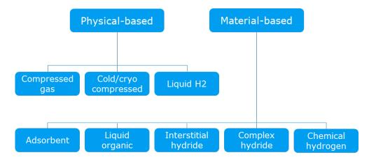
Figure 7 Different options to store hydrogen. Developed from [10].
