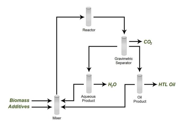
Figure 1 Hydrothermal Liquefaction Process Flow
