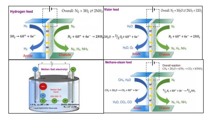
Figure 10. Illustration of the anode and cathode reactions during electrochemical NH<sub>3</sub> production. [1]
