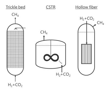
Figure 7. Examples of reactor design for biological methanation
