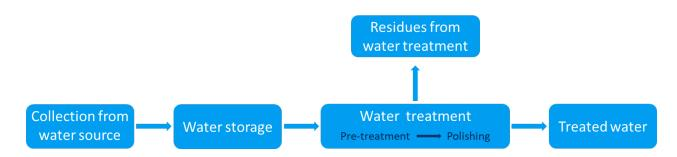
Figure 6 General flow diagram of water.
