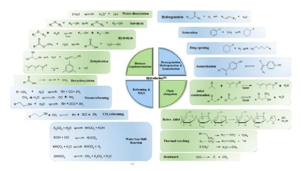
Figure 3 Major Chemical Reactions in the Steeper Energy Process
