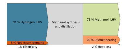
Figure 3: Energy balance of a methanol plant.
