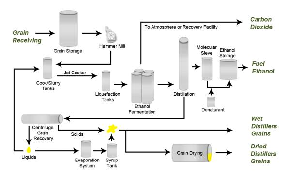
**Figure 1 1st Generation Ethanol Production Process**
