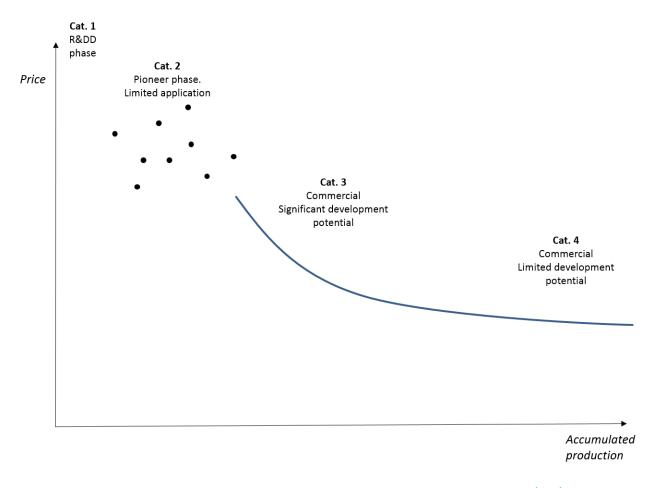
Figure 9: Technological development phases, correlation between accumulated production volume (MW) and price.
