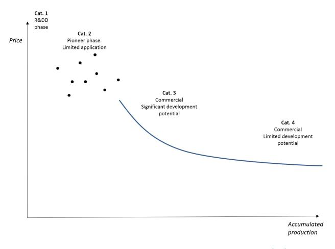
Figure 2: Technological development phases, correlation between accumulated production volume (MW) and price.
