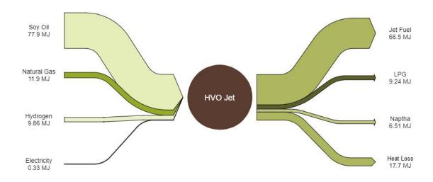
Figure 2 HVO Jet Fuel Energy Balance
