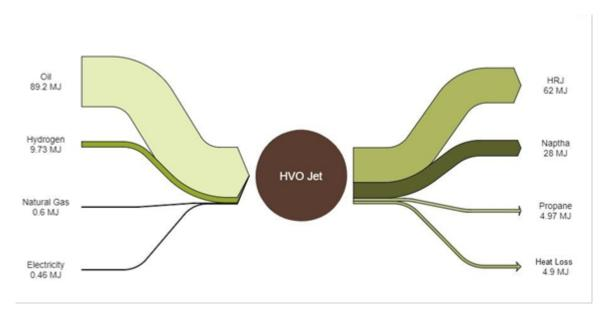
Figure 4 Alternative HVO Jet Energy Balance
