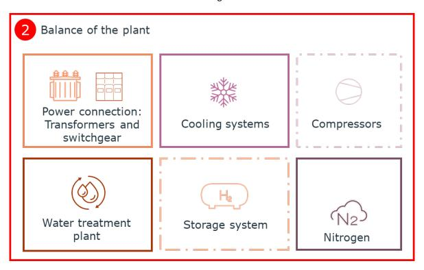
Figure 5 General components of the balance of the plant in a H<sub>2</sub> plant. Compressors and storage system are shown with dotted lines as they are not required in every hydrogen plant.
