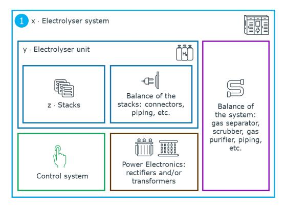
Figure 3 Schematic of the different components included in an electrolyser system: electrolyser units, balance of the system, power electronics and control system.
