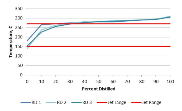
**Figure 5 Renewable Diesel Distillation Curves**
