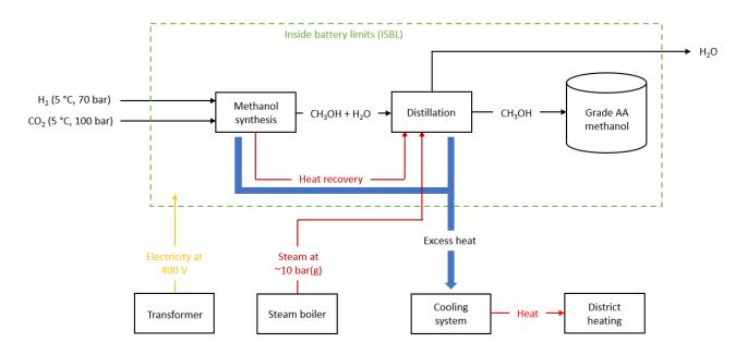
Figure 5: Illustration of battery limits.
