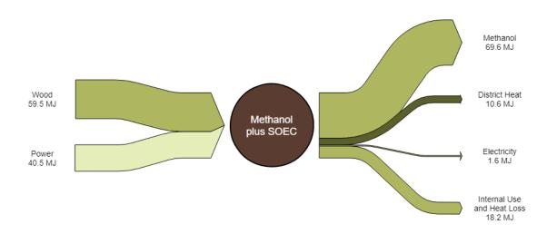
**Figure 5 Hybrid Biomass to Methanol Plant**
