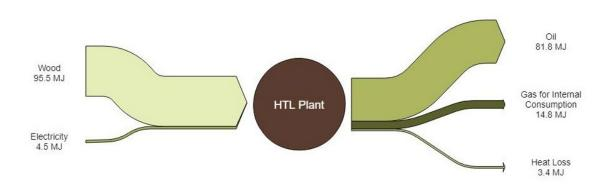
Figure 2 Hydrothermal Liquefaction Energy Balance
