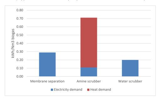
Figure 12: Energy consumption (kWh/Nm³ raw biogas) for the upgrading technologies, water scrubbing, amine scrubber and membrane
