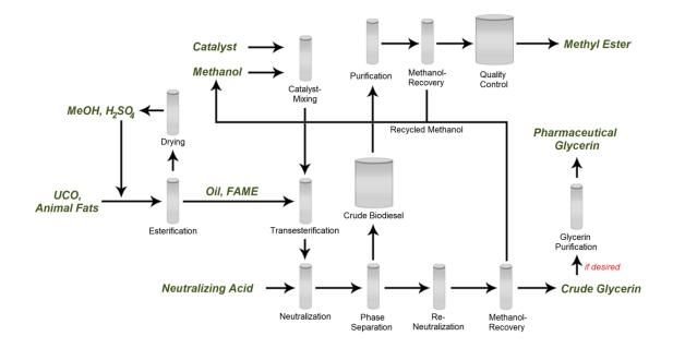
**Figure 1 Two Step Biodiesel Production Process**
