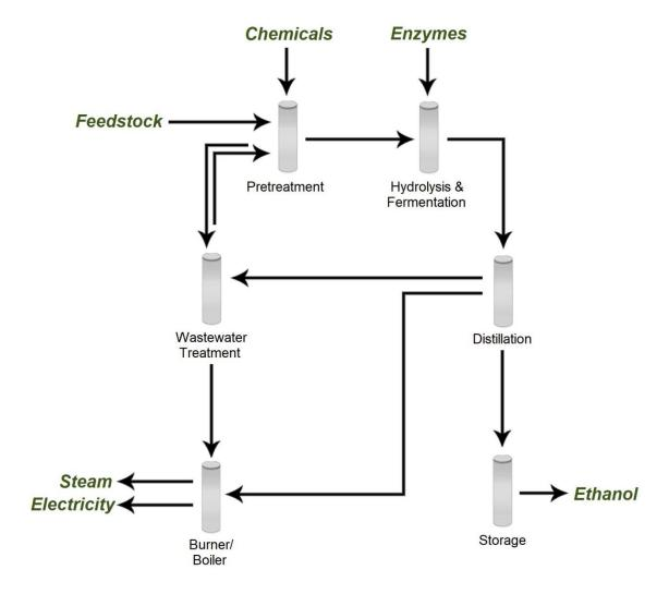
**Figure 1 Cellulosic Ethanol Process**
