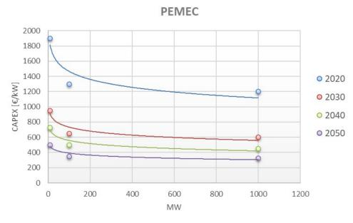
Figure 15 CAPEX of electrolyser plant, based on scale and time for PEMEC.
