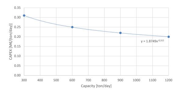
Figure 4: CAPEX as a function of capacity.
