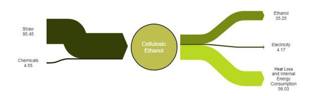
Figure 3 Cellulosic Ethanol Energy Balance with Chemicals
