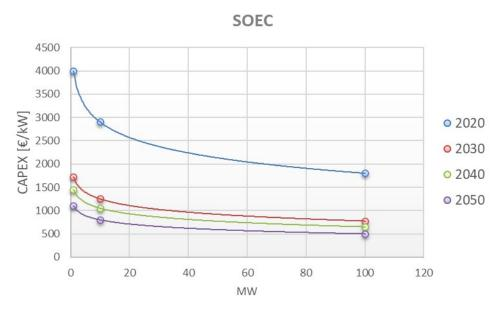
Figure 16 CAPEX of electrolyser plant, based on scale and time for SOEC.
