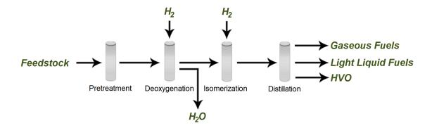
**Figure 1 HVO Production Process**
