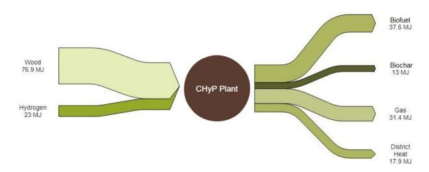
Figure 2: Catalytic Hydropyrolysis Energy Balance – Configuration 1
