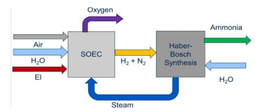
Figure 11: SOC4NH3 project combining electrolysis unit and ASU (El = power)[ref 15]
