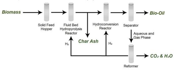
Figure 1: Catalytic Hydropyrolysis Process Flow
