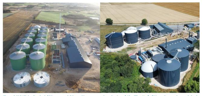
Figure 8 SBS Kliplev (to the left) is approx. 8.5 ha and has an annual production of 48 million Nm³ of biomethane, whereas Solrød biogas (to the right) is approx. 2 ha and has an annual production of 11 million Nm³ biomethane [23, 21]
