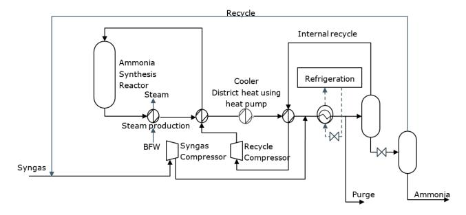
Figure 8: Ammonia synthesis loop and downstream purification
