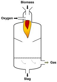
Principle of the entrained flow gasifier.
