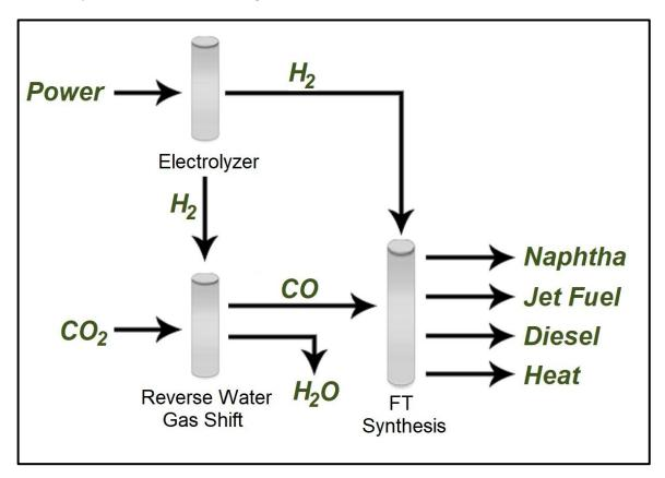
Figure 1: Power to Jet Process Flow
