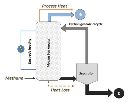
Figure 3. Thermal-assisted (moving-bed reactor) Decomposition Diagram.
