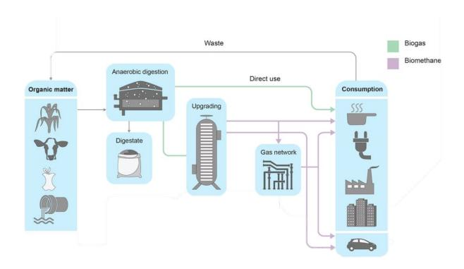
Figure 10: Biogas may either be used directly as an energy source or be upgraded through an upgrading plant to be fed into the gas network or be directly applied for consumption needing gas with high energy content. Illustration from IEA [2]
