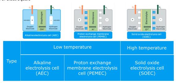
Figure 4 The three primary electrolyser technologies: AEC, PEMEC, and SOEC.
