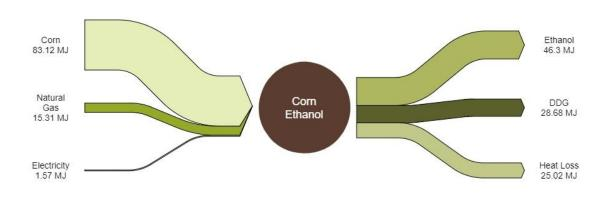
Figure 2 1st Generation Ethanol Energy Balance
