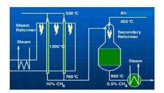
Figure 4: Primary and secondary reformer arrangement
