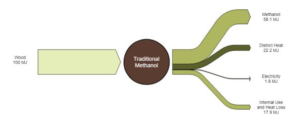
Figure 3 GreenSynFuels Traditional Methanol Plant
