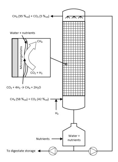
Figure 5: Sketch of a "trickle bed" biomethanation reactor. CSTR reactors have also been developed to near maturity (not shown).
