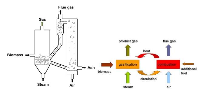
The dual CFB (circulating fluidised bed) process (Güssing type design) [14]
