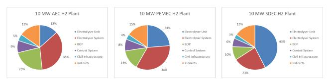
Figure 17 Cost breakdown of a 10 MW hydrogen plant for (left) AEC, (middle) PEMEC, and (right) SOEC.
