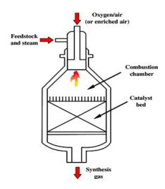
Figure 5: Autothermal reformer (ATR)
