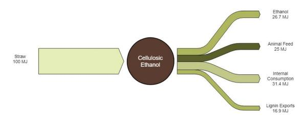
Figure 4 Inbicon Cellulosic Ethanol Energy Balance
