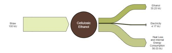
Figure 2 Cellulosic Ethanol Energy Balance
