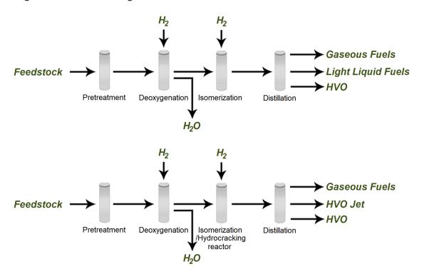
Figure 1 HVO Diesel vs Jet Process
