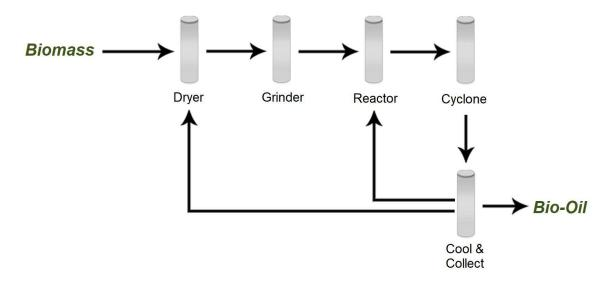
Figure 1 Fast Pyrolysis Process Flow
