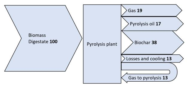
Figure 4. Example of energy balance for slow pyrolysis of digestate from biogas production, 20% incoming moisture content. All inputs sum to 100 units. Note, the balance shows the core process only. Assumed pyrolysis temperature is 550-600°C. The gas to pyrolysis stream can be seen as an internal stream in the pyrolysis plant, as a fraction of the output gas is recirculated into the pyrolysis process.
