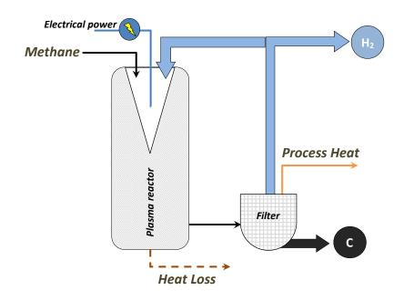
Figure 4. Plasma-assisted Decomposition Diagram.
