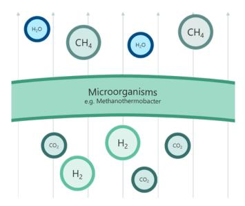
Figure 2: Microorganisms in a biomethanation process where hydrogen and carbon dioxide react to form methane and water.
