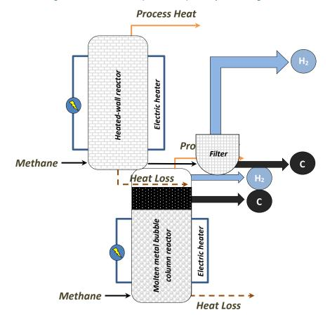
Figure 1. Thermal-assisted (heated-wall) Decomposition Diagram.
