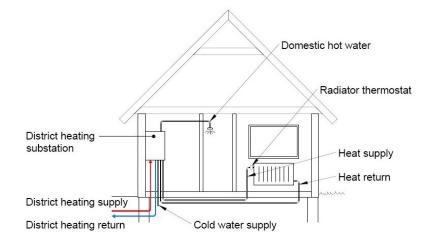
Figure 9: District heating substation with domestic hot water heater and heat exchanger for space heating
