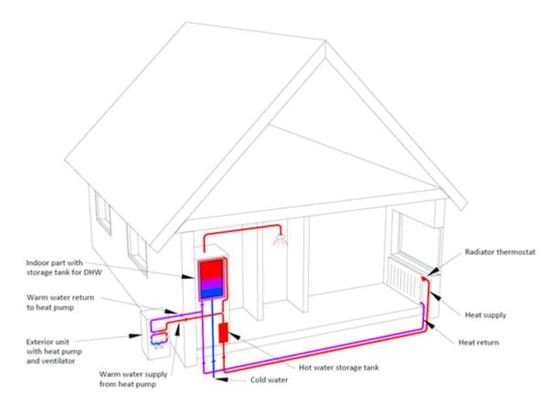
Figure 3: Air-to-water heat pump
