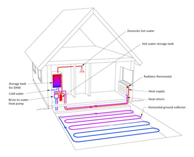
Figure 4: Ground-source heat pump (brine-to-water)
