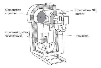
Figure 5: A floor standing medium size condensing gas boiler for apartment blocks etc. (Source: VarmeStåbi<sup>®</sup>, Nyt Teknisk Forlag)
