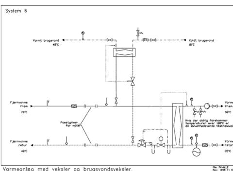
cities, more than 95% of the end users are typically connected to the district heating system. District heating units are categorised ลร either direct or indirect units. The district heating substation is placed at the end user with the purpose of preparing domestic hot water and delivering heat for the space
