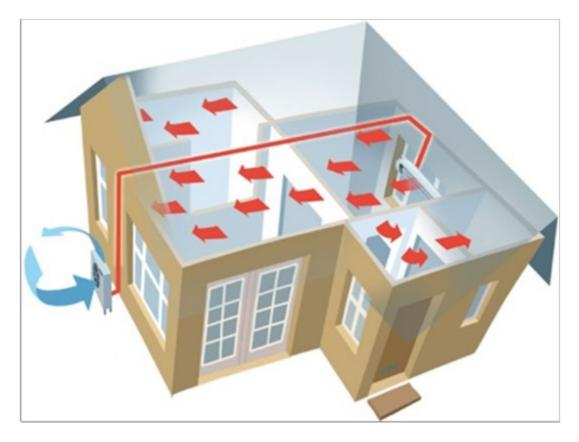
Figure 2: Air-to-air heat pump. The two units are placed according to concrete local conditions.
