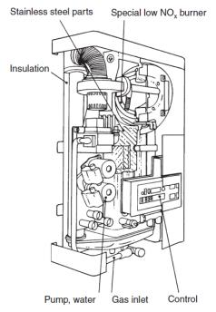
Figure 4: A wall hung gas boiler for a one-family house (Source: VarmeStåbi®, Nyt Teknisk Forlag)
