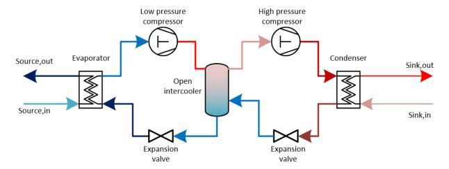
Figure 1: Sketch of two-stage compression heat pump
