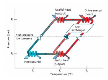
Figure 1: Principle of operation, heat driven heat pump, edited from [3]
