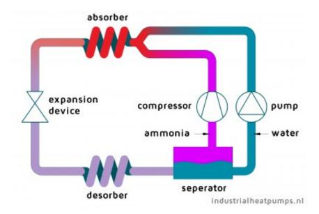
Figure 1: Simplified hybrid absorption-compression heat pump
