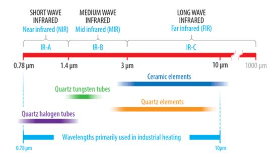
Figure 2: Infrared subdivisions and types of infrared element for different wave length
