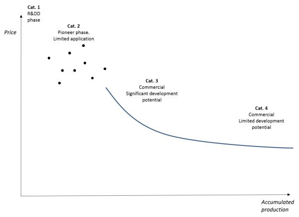
Figure 3: Technological development phases. Correlation between accumulated production volume (MW) and price.
