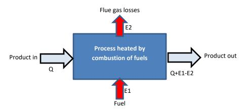
Figure 5: Energy balance of a direct firing process.
