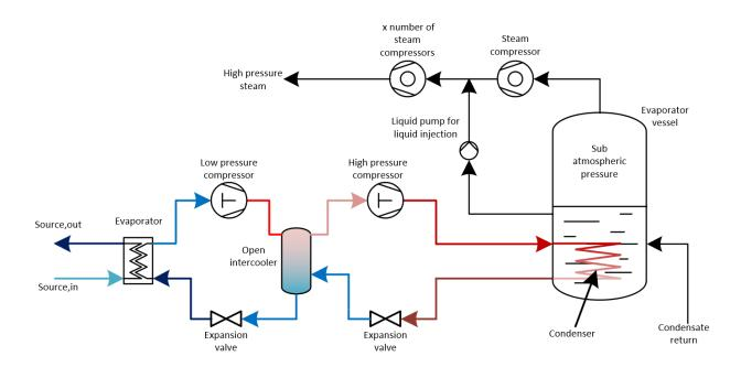
Figure 1: Sketch of two-stage compression heat pump in combination with booster turbo compressors. Components and process is described in detail above.
