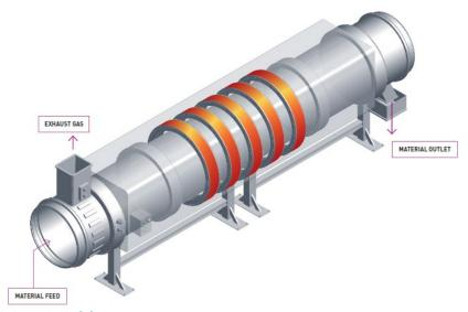
Figure 4: Electrically heated Kiln [9].
