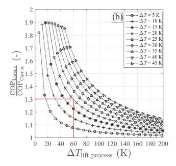
Figure 2: Theoretical advantage of using a HACHP compared to a normal vapour compression heat pump, as a function of temperature lift (x-axis), and glide [4].  $\Delta T_{Lift,proces} = \text{Sink outlet}$  - Source inlet
