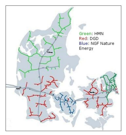
Figure 2 Geographical extent of the Danish transmission network (grey) and the main distribution network (green, red & blue). The colours refer to the companies operating the system.
