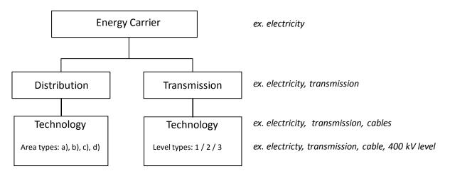
With a view to cross-technology comparisons, a general separation between transmission and distribution systems is maintained throughout the catalogue, as defined below. Thus, an entire energy transport system for a specific energy carrier may consist of a combination of transmission technologies and distribution ones.
