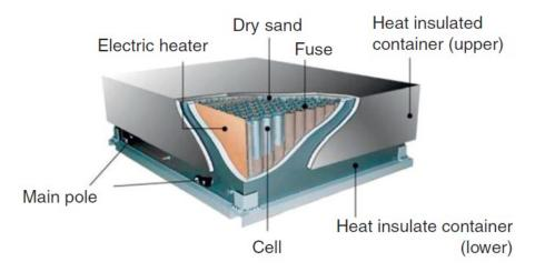
Figure 3: Illustration of Na-S battery module. [4]
