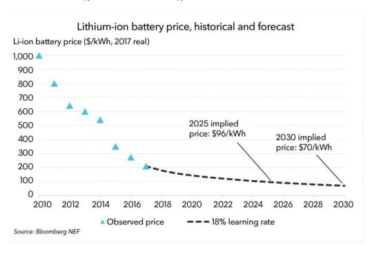
Figure 8: Historical and forecasted Lithium-ion battery pack cost [44].
