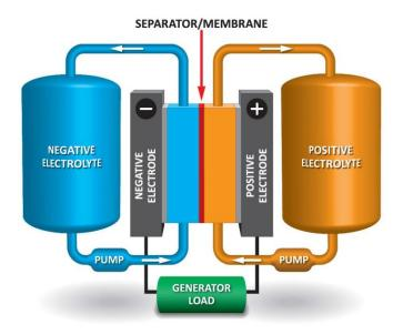
Figure 1: Schematic of flow battery [1].
