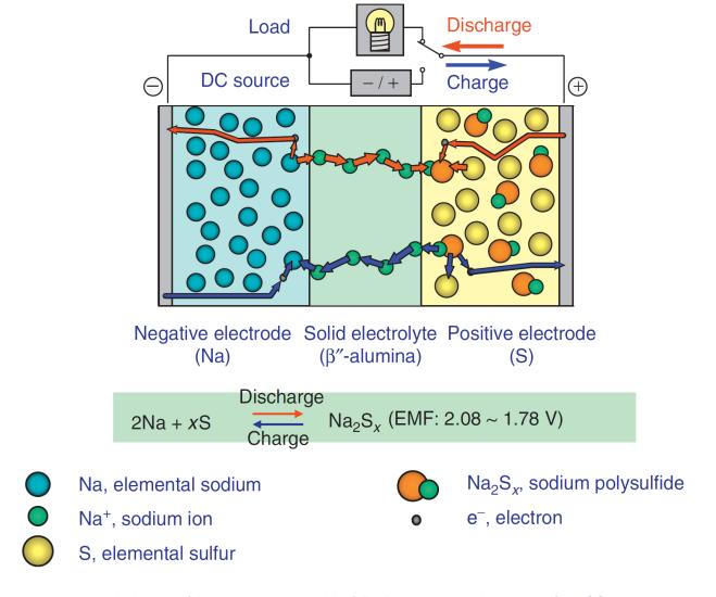
Figure 2: Graphical schematic of the reaction process and the full cell reaction. EMF: electromotive force. [4]
