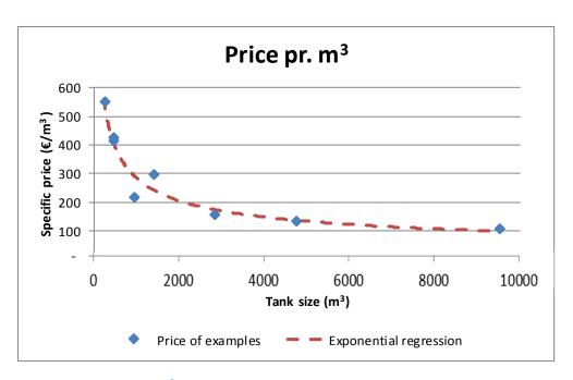
Figure 3: Specific price pr. m³ by total size of tank, incl. foundation [2 & 4].
