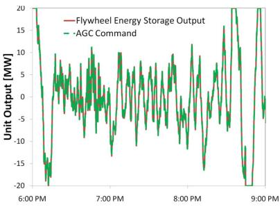
Figure 4: The reaction of a flywheel (MW input/output) in response to signals from the Automatic Generation Control. It can be seen that within the accuracy of the graph (please note the axis scaling) the flywheel follows signals completely. Source: Beacon Power.
