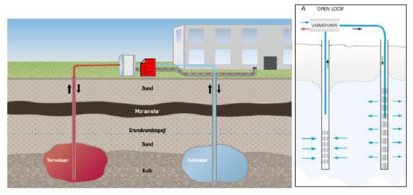
Figure 6: Principle of an ATES [1].
