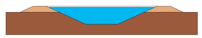
Figure 2: Principle sketch of a pit heat storage cross section [15].
