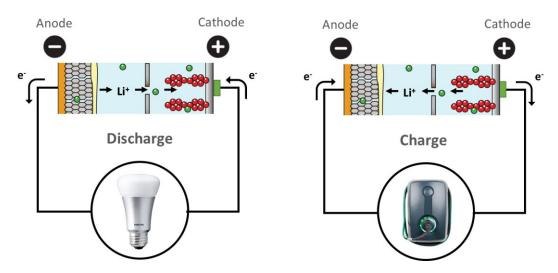
Figure 2. Schematic diagram of a LIB system in charge and discharge mode. During discharge the green Li+ ions moves from the negative electrode (left side) to the positive electrode. The process is reversed during charge mode (right side).
