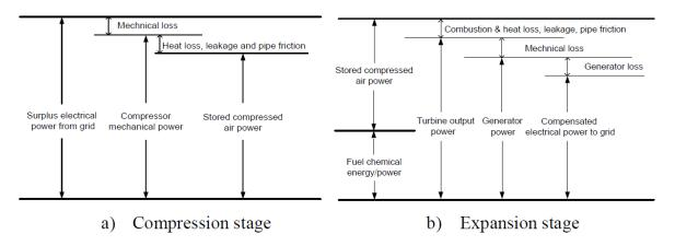
Figure 4: Energy transfer of a conventional CAES plant [7]. The source does not quote numbers but only graphics.
