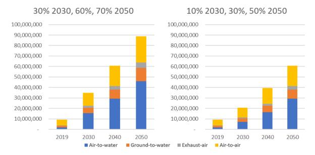
Figure 43: Number and type of heat pumps in the 2 scenarios
