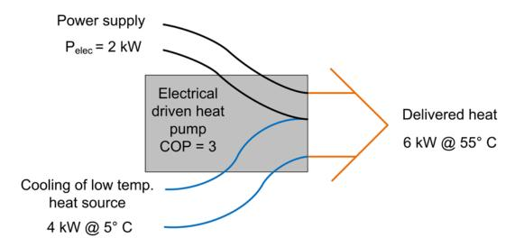
Figure 31 Sankey diagram for a heat pump.
