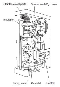
Figure 7 A wall hung gas boiler for a one-family house (Source: VarmeStåbi®, Nyt Teknisk Forlag)
