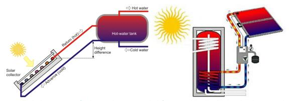
Figure 45: Small solar heating system for domestic hot water. To the left a pumped system where auxiliary heat is supplied to the upper heat exchanger coil. To the right a thermosyphon system without pump. In such a system the circulation of the heat transfer fluid is driven by natural convection rather than a mechanical pump. By far the most systems are equipped with a pump.
