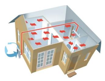
Figure 34 Illustration of a heating system based on a ventilation heat pump.
