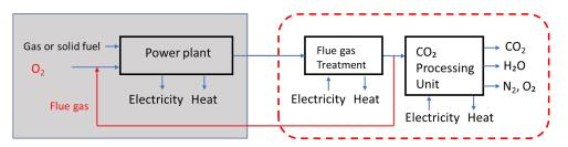
Figure 7: Oxy-fuel combustion
