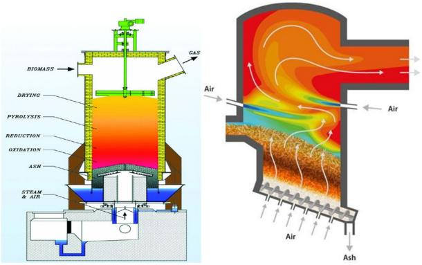
Figure 1: Simplified illustration of Vølund's (left) and Dall Energy's (right) Up Draft gasification equipment
