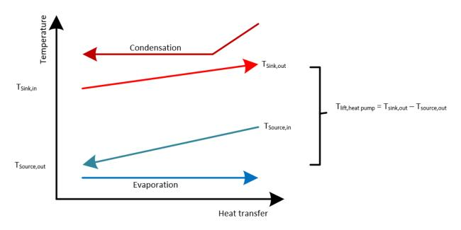
Figure 2: Q-T diagram depicting heat transfer in evaporator and condenser. Includes heat pump temperature lift
