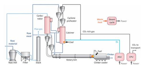
Figure iii-5. Partial oxy-fuel combustion with integrated Calcium looping (49)
