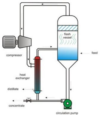
Figure 1: Simplified illustration of the MVR cycle. For a water treatment system, the feed is dirty water, the concentrate is highly concentrated pollutants, and the condensate/distillate is pure water.
