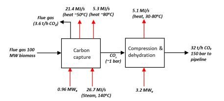
Figure ii-2. Illustration of energy balance for a  $CO_2$  capture and compression plant treating all flue gas from a 100 MW<sub>th</sub> biomass boiler that is equipped with flue gas condensation. 90% of the  $CO_2$  in the flue gas is captured corresponding to 32 t  $CO_2$  output per hour. Black arrows: Mass streams. Red arrows: Energy streams.
