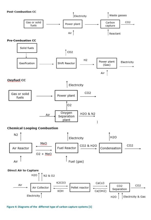
The first three system types resemble the more traditional power plant solutions and has been proven at a larger scale, while Chemical looping combustion is only at demonstration scale and could be seen as a special case of oxy-fuel combustion. Direct Air to Capture (DAC), however distinguish itself significantly from the other four technologies, as its sole purpose is to capture CO<sub>2</sub> and not limit the emissions from power and heat production.[1]
