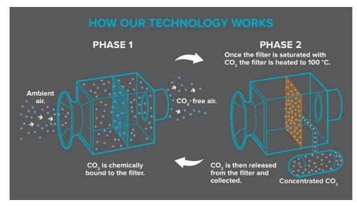
Figure iv-1. Illustration of working principle of Climeworks low temperature adsorption DAC process. Source: www.climeworks.com
