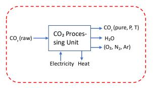
Figure 9. Illustration of CO<sub>2</sub> processing (conditioning) unit.
