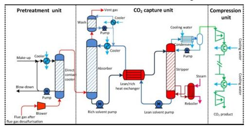
Figure ii-1. Schematic illustration of amine based  $CO_2$  capture process as reported in [11]. Flue gas is cooled in a pretreatment unit prior to entering the  $CO_2$  capture unit where  $CO_2$  is washed out by an amine solution. The  $CO_2$  gas is stripped of the amine solution whereby it is regenerated by applying heat in a stripper (desorber). The recovered  $CO_2$ may be compressed and dehydrated for transportation.
