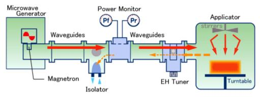
Figure 1: Schematic drawing of microwave system [7]
