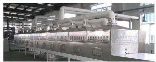
Figure 3. Industrial microwave heating system (Max Industrial Microwave)
