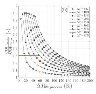
Figure 2: Theoretical advantage of using a HACHP compared to a normal vapour compression heat pump, as a function of temperature lift (x-axis), and glide [4].  $\Delta T_{Lift,proces}$  = Sink outlet - Source inlet
