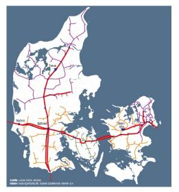
Figure 5. Natural gas pipeline network (steel piping) in Denmark. Source: Naturagasfakta.dk, DGC.
