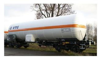
Figure 8. Railroad car for liquid CO<sub>2</sub> transport. Source: www.VTG.com
