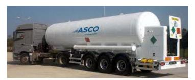
Figure 7. CO<sub>2</sub> semi-trailer from ASCO. Source; www.ascoco2.com
