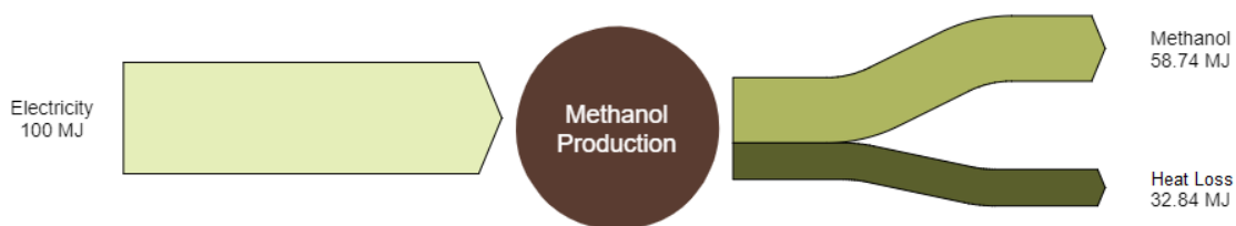
Figure 2 Methanol from Power Energy Balance
