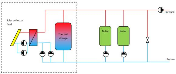
Figure 11 Schematic drawing of a possible system integration of solar district heating [5].
