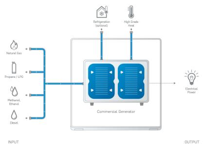
Figure 2: Schematic illustration of an SOFC unit for combined heat and power for commercial use from Sunfire illustrating the flexibility in input fuels [9].
