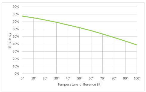
Figure 10 Efficiency as a function of temperature difference. (Based on data from [8], example with G=1.000 W/m<sup>2</sup>,  $\eta_0$ =0.777,  $a_1$ =2.41,  $a_2$ =0.015)<sup>20</sup>
