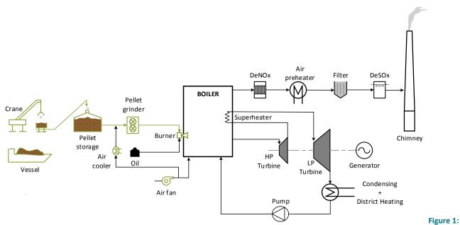
Sketch of a CHP plant converted to firing with wood pellets. The green elements indicate the equipment that needs to be added, replaced or refurbished.
