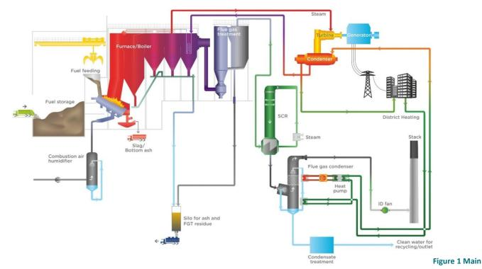
systems of a CHP (or Heat only) facility, example WtE CHP facility
