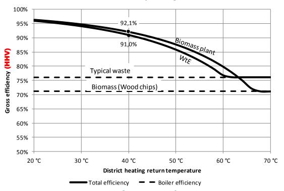
Figure 7. Total HHV-based efficiency estimate for WtE plants<sup>7</sup> and biomass plants<sup>8</sup> given varying DH return temperatures [5] – or temperature of the cold media of a heat pump.
