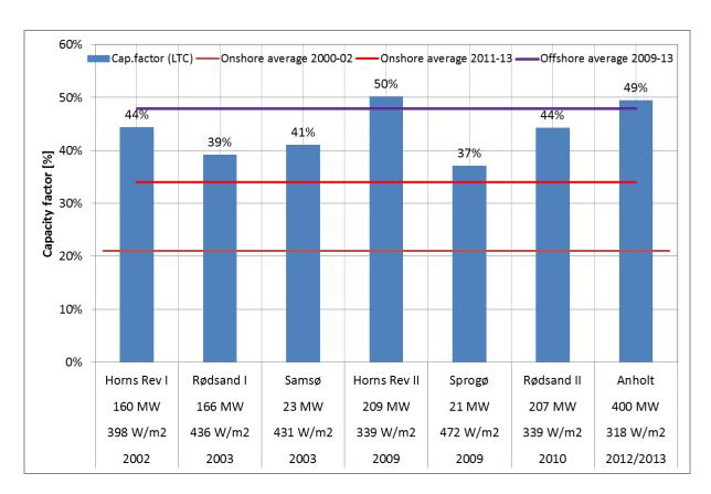
Figure 4: Long term corrected (LTC) capacity factors for five large offshore wind farms (>150 MW) and two smaller offshore wind farms located nearshore in Denmark. For comparison is shown the average capacity factor for onshore turbines installed 2000-02 and 2011-13 based on measured 2014 performance (which was a normal wind year) [8]. Year of commission shown in graph.
