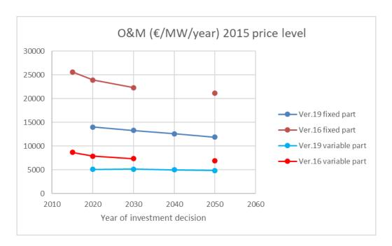
Figure 21 Expected O&M cost, divided into fixed and production dependent (variable, app. 25% of all O&M costs)
