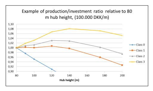
Figure 14 The production increase relative to the investment cost based on current available Vestas turbines. By increasing height, costs are extrapolated using DKK 100.000 per m hub height increase; the rotor area is kept constant.
