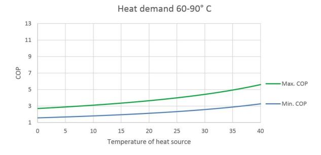
Figure 5: COP values of compression heat pump heating water from 60 to 90° C. For a heat source @ 0° C that is cooled to -5° C, typical COP values will be 1.6-2.7 rising to 3.2-5.6 for a heat source @ 40° C that is cooled to 35° C [1].
