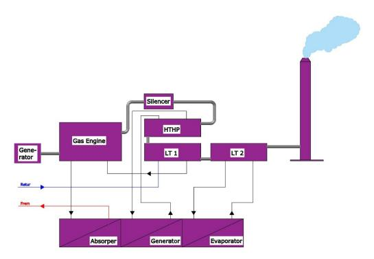
Figure 1 A gas engine based cogeneration unit with heat recovery boilers and an absorption heat pump to obtain a high heat production and highest possible overall efficiency. The heat pump is steam driven [9].
