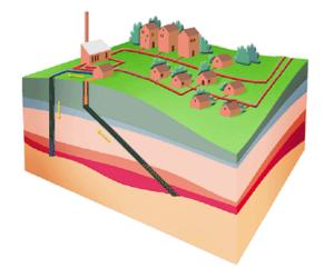
Figure 1: The principle of a doublet system [7]
