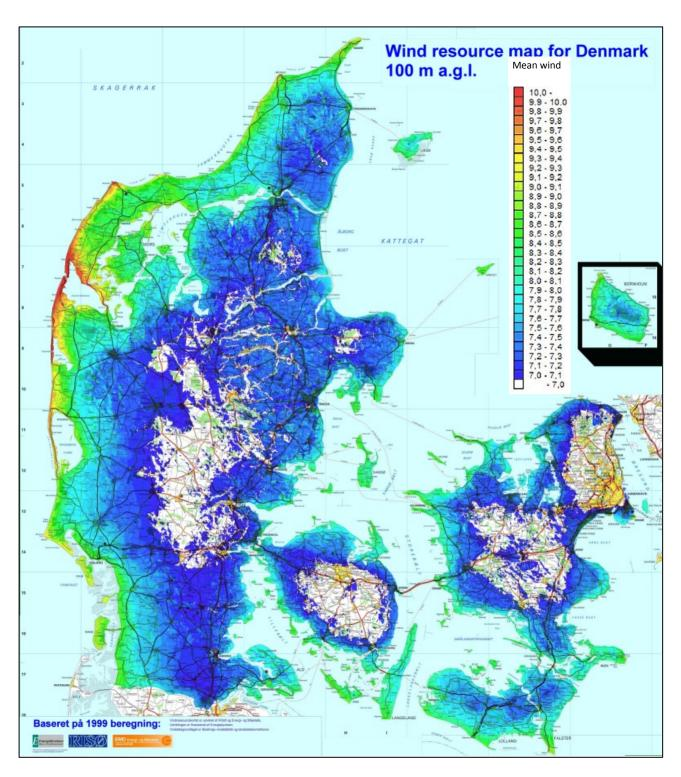
Figure 6 Wind resource map for Denmark in 200 m resolution, 100 m above terrain .
