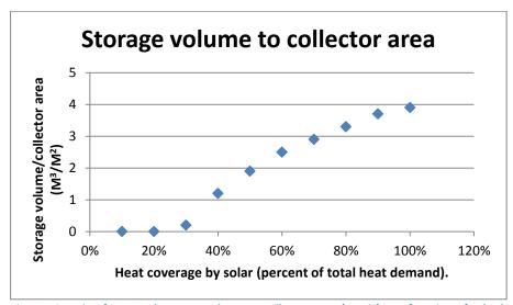
Figure 18 Ratio of seasonal storage volume to collector area (y-axis) as a function of solar heat coverage [4] and [5].
