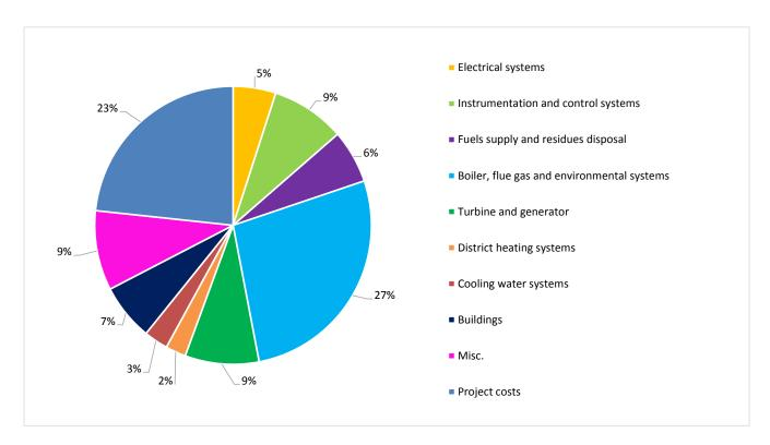
Figure 2: Diagram showing an example of the share of investment cost for an LTE project.
