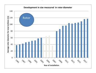
Figure 9 Average rotor diameter for new turbines (rated power > 25 kW) [3]
