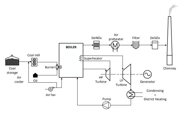
Figure 1: Sketch of the main elements of a large coal fired CHP plant.
