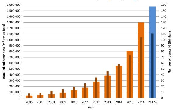
Figure 14 Solar district heating plants in Denmark in operation (until 2017) and planned. The trend is that the new plants are larger and include seasonal heat storages [5].
