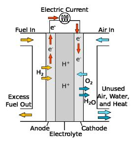
Figure 1: Diagram of a PEM-FC [2].
