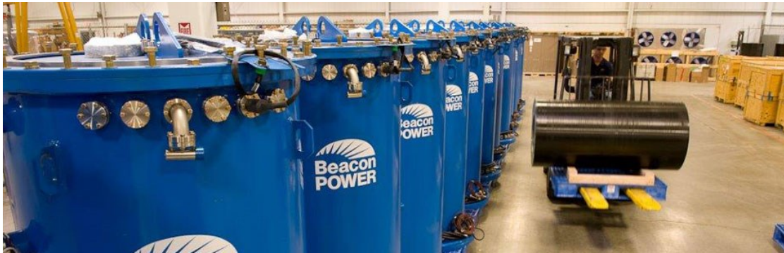
Figure 2: Photo of Beacon Power’s flywheels [6]. The fiber composite flywheel itself is seen to the right on the fork-lift. Each unit is 100 kW. Photo from manufacturer’s store.
