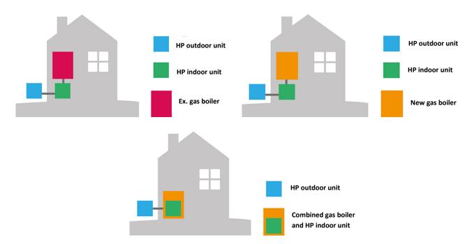
Figure 45: Principle of the three hybrid heat pump solutions. Left to right: add-on, package, and integrated solution [2]
