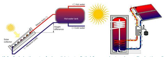
Figure 49: Small solar heating system for domestic hot water. To the left a pumped system where auxiliary heat is supplied to the upper heat exchanger coil. To the right a thermosyphon system without pump. In such a system the circulation of the heat transfer fluid is driven by natural convection rather than a mechanical pump. By far the most systems are equipped with a pump.
