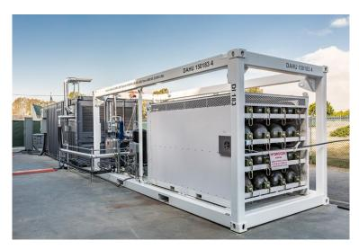
Figure 2: SOEC hydrogen plant from Sunfire [11].
