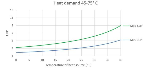
Figure 4: COP values of compression heat pump heating water from 45 to 75° C. For a heat source @ 0° C that is cooled to -5° C, typical COP values will be 2.0-3.1 rising to 5.0-9.0 for a heat source @ 40° C that is cooled to 35° C [1].
