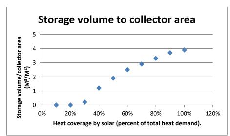
Figure 11 Ratio of seasonal storage volume to collector area (y-axis) as a function of solar heat coverage [4] and [5].
