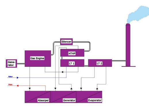
Figure 1 A gas engine based cogeneration unit with heat recovery boilers and an absorption heat pump to obtain a high heat production and highest possible overall efficiency. The heat pump is steam driven [9].
