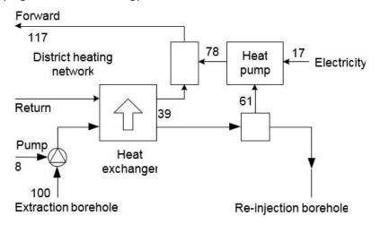
Figure 5: Example of a system with an electric heat pump. The COP of the electric heat pump is approximately 4.6 and the COP of the total system is approximately 4.7.
