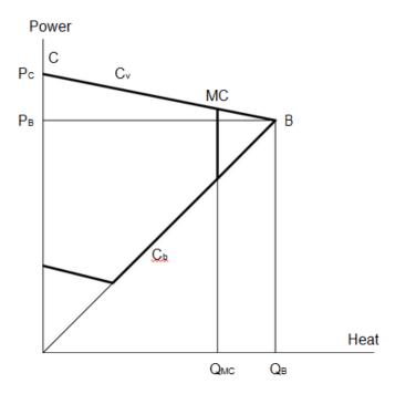
With the steam boiler at full capacity, the turbine may be operated at all points along the line C-B. In the real world, C-B may not be a straight line, but a linear relationship is a good proxy.
