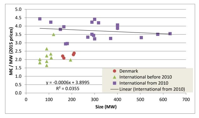
Figure 9: Cost plotted against farm size for 35 realized offshore projects in DK, UK, DE and SE from 2002 to 2014.
