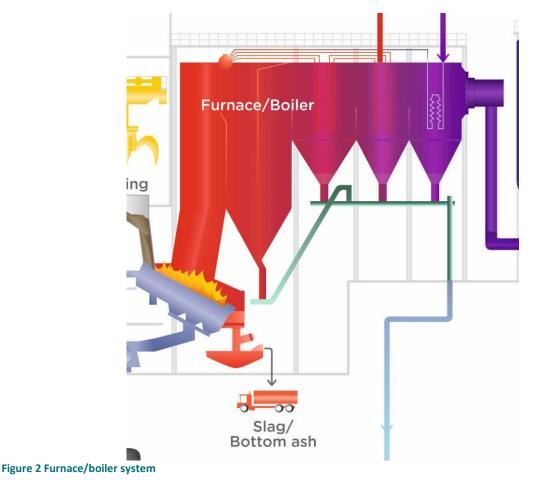
The output from the boiler of a CHP facility is superheated steam, i.e. steam that is heated above the boiling point. The plant includes feed water pumps supplying high pressure water to the boiler, an economiser, where the input water is heated towards the boiling temperature, evaporators, where the water is
