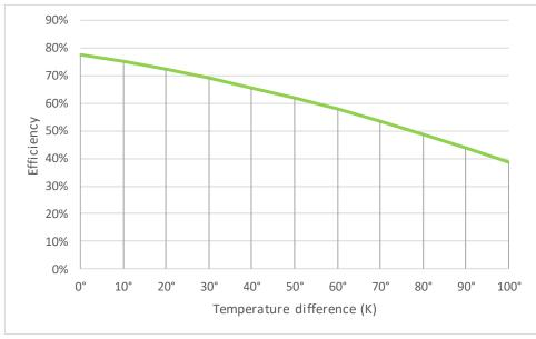
Figure 3 Efficiency as a function of temperature difference. (Based on data from [8], example with G=1.000 W/m<sup>2</sup>,  $\eta_0$ =0.777,  $a_1$ =2.41,  $a_2$ =0.015)<sup>20</sup>
