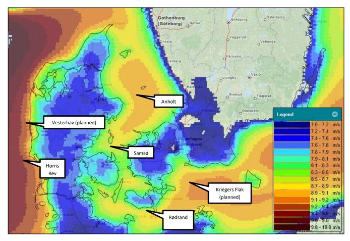
Figure 1 Wind resource map for Denmark (height above terrain/sea level: 75 m) based on EMD-ConWx meso scale modelled wind data [1]
