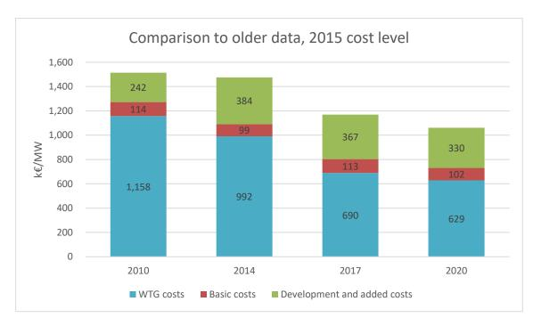
Figure 18 Development in average costs for "Køberets" projects together with 2020 estimate. Basic is foundation, roads and internal grid, the needed "hardware" in addition to the turbines. Development and added costs cover land rent, neighbor compensations and purchase of neighbour settlements and old turbines if such on the site or nearby. Grid connection costs are not included.
