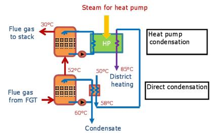
Figure 5 Flue gas condensation, direct and heat pump driven with 50°C DH return temperature, and typical WtE adiabatic scrubber temperature of 60°C.
