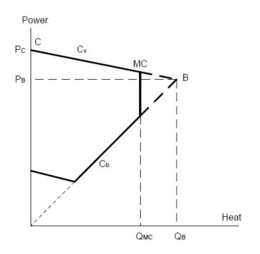
Pc: Power capacity in full condensation mode; point C. No heat production.
