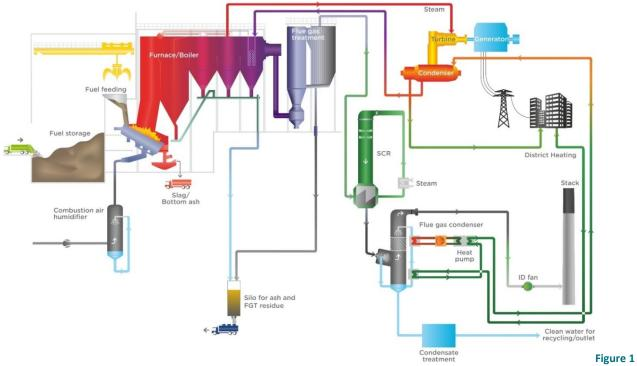
Main systems of a CHP (or Heat only) facility, example WtE CHP facility
