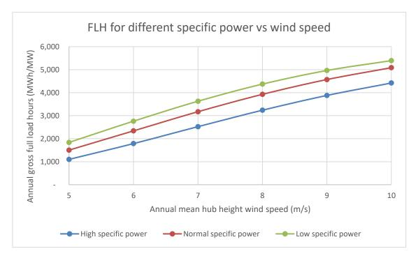
Figure 7 Annual full load hours as a function of mean wind speed at hub height. The examples in the figure are 3 MW with 90m rotor diameter, specific powers are 472 W/m2 called "high specific power" and 3.3 MW turbines with 112 m and 126 m rotor diameters, specific powers are 335 W/m<sup>2</sup> called "medium specific power" and 265 W/m<sup>2</sup> called "low specific power".
