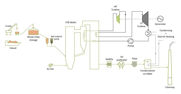
Figure 2: Sketch of a CHP plant converted to firing with wood chips with a new CFB boiler. The green elements indicate the equipment that needs to be added, replaced or refurbished.
