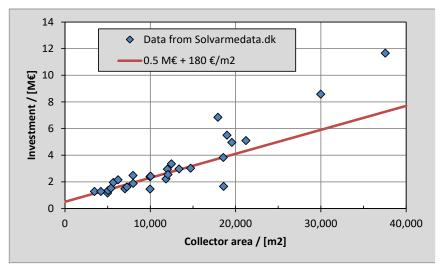
Figure 10 Solar plant investment for Danish SDH projects. The plant in the upper right corner is "Dronninglund" with 37,573 m2 which includes a seasonal heat storage – and the investment for that is 2.4 M€ (see the section below on the seasonal heat storage), bringing this plant closer to the red line [5].
