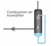
Figure 6 Combustion air humidifier, where water heated by a low-temperature source is evaporated into the combustion air flow.
