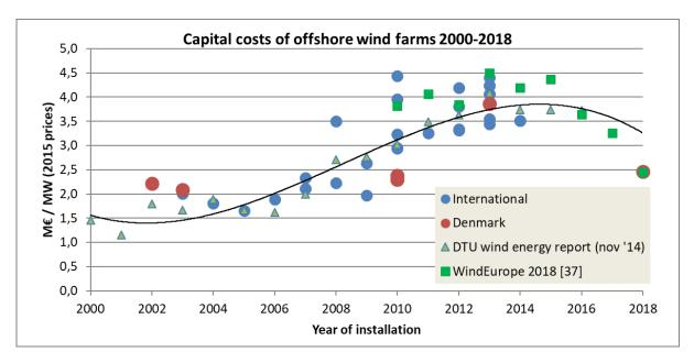
Figure 10: Capital costs for offshore wind farms. EMD graph based on data from [10, 15, 16]. The dot is placed at the first year in operation. Cost includes substation and land cable [10] and is annual averages based on selected projects and includes prognoses for 2015-16. The latest Danish project Horns rev III is not included in the graph.
