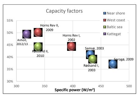
Figure 5: Capacity Factor shown as function of the Specific Power (W/m<sup>2</sup>) for Danish Offshore wind turbine projects. The 3 most left are the latest projects.
