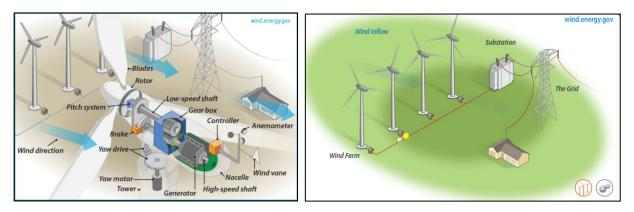
Figure 2 General turbine technology and electrical system.
