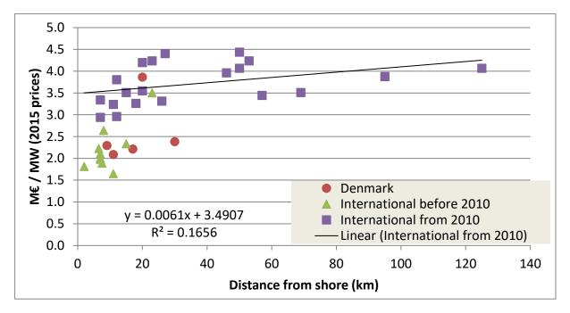
Figure 8: Cost plotted against distance to shore for 35 realized offshore projects in DK, UK, DE and SE from 2002 to 2014.
