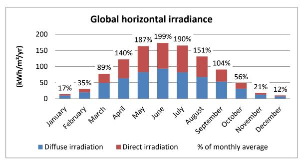
Figure 1: Monthly sum of global irradiance on a horizontal surface averaged over 25 Danish measurement stations over a period of 10 years (2001-2010) (Ref 4). The split between direct and diffuse components of the irradiation is based on the Meteonorm '97 dataset for Copenhagen. Percentage of average monthly is also shown.
