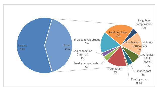
Figure 13 The cost breakdown including land costs etc. from "køberetsordning" 2017-18 projects.
