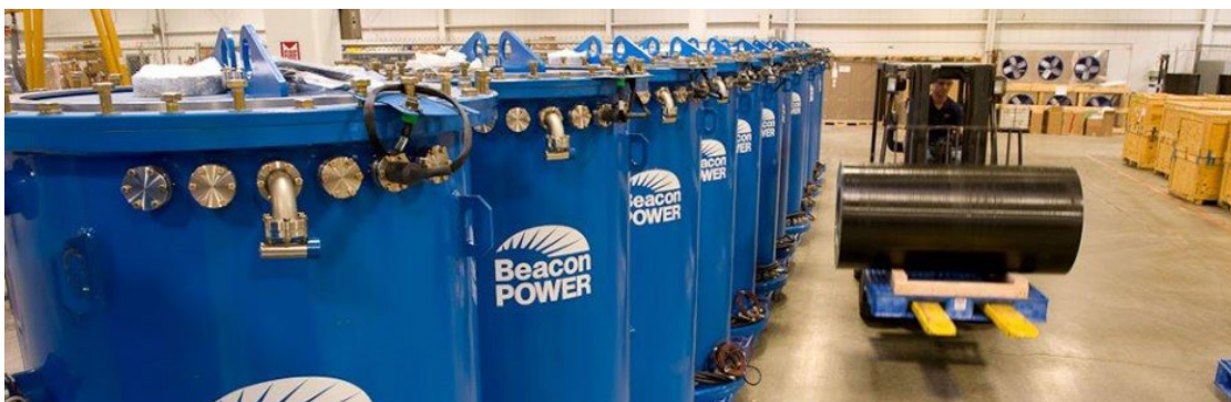
Figure 2: Photo of Beacon Power's flywheels [6]. The fiber composite flywheel itself is seen to the right on the fork-lift. Each unit is 100 kW. Photo from manufacturer's store.
