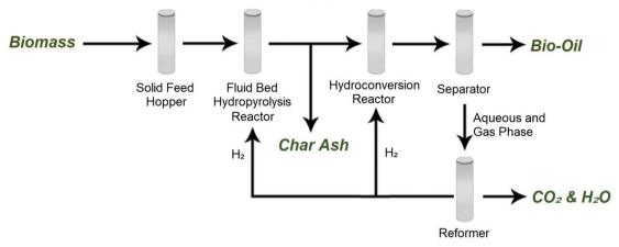
Figure 1: Catalytic Hydropyrolysis Process Flow
