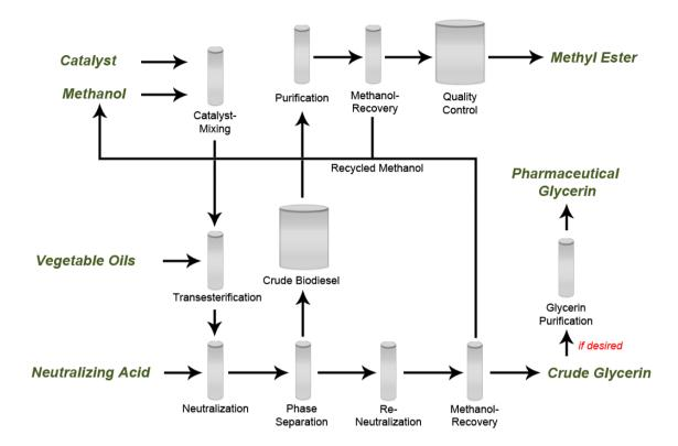
**Figure 4 Biodiesel Production Process**
