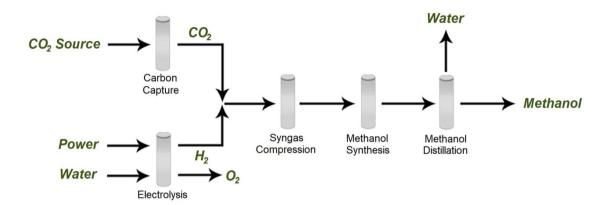
**Figure 1 Methanol to Power Process**
