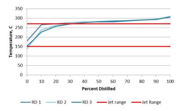
**Figure 5 Renewable Diesel Distillation Curves**
