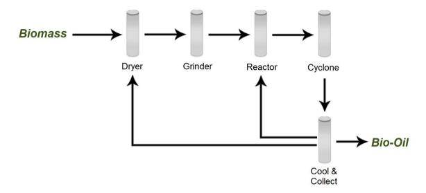
Figure 1 Fast Pyrolysis Process Flow
