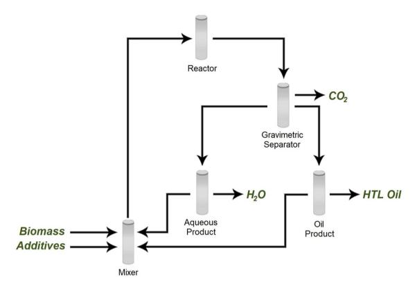
Figure 1 Hydrothermal Liquefaction Process Flow
