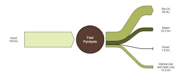
Figure 2 Fast Pyrolysis Oil Energy Balance
