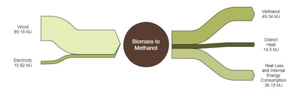
Figure 2 Bio Methanol Energy Balance
