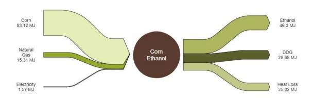
Figure 2 1st Generation Ethanol Energy Balance
