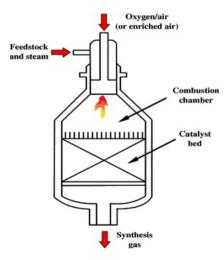
Figure 5: Autothermal reformer (ATR)
