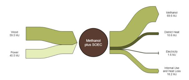
Figure 5 Hybrid Biomass to Methanol Plant
