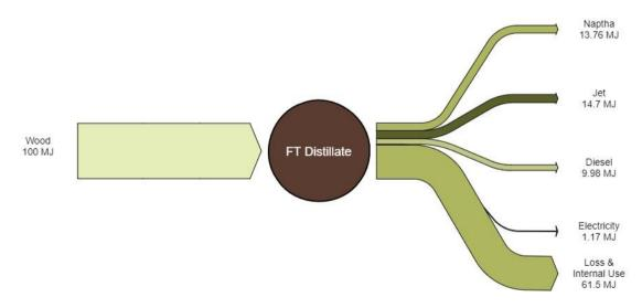
Figure 2 Biomass to Diesel and Jet Energy Balance
