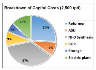
Figure 15. Cost split on main systems in a conventional NH<sub>3</sub> plant from Linde [10]. Reformer, electric plant (power plant) and some balance of plants (BOP) will disappear for a green NH<sub>3</sub> plant. Cost of green NH<sub>3</sub> plant (excl. electrolysis unit and ASU) is therefore taken as 54% of conventional plant, based on all obtained data.
