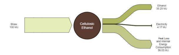
Figure 2 Cellulosic Ethanol Energy Balance
