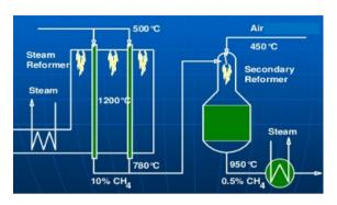
Figure 4: Primary and secondary reformer arrangement
