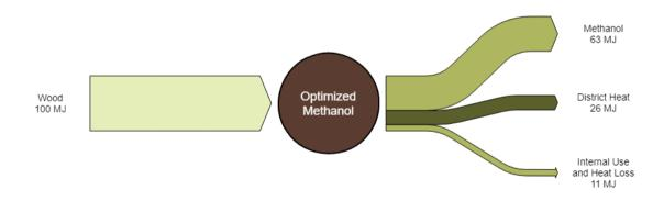
**Figure 4 Optimized Biomass to Methanol Plant**
