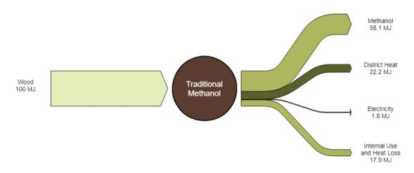
Figure 3 GreenSynFuels Traditional Methanol Plant
