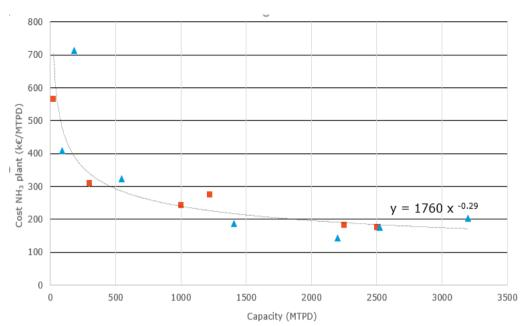
Figure 16: Estimated cost of ammonia synthesis + BOP + Storage (electrolysis unit and ASU is not included in the figure). Blue triangles represent data that is publicly available. All figures adjusted to reflect cost index for 2019.
