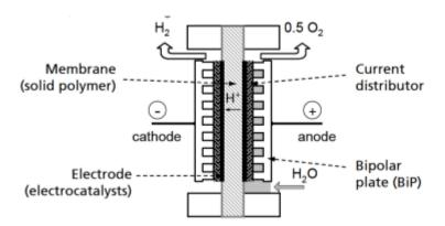
Figure 1: Principle of a PEMEC. Adopted from [13]
