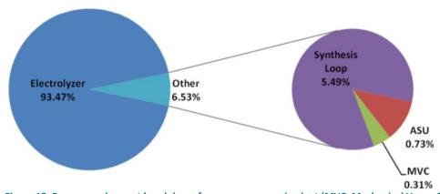
Figure 13: Power requirement breakdown for a green ammonia plant (MVC=Mechanical Vapor Compression, includes pumping and desalination of feed water to electrolysis unit) [ref 7].
