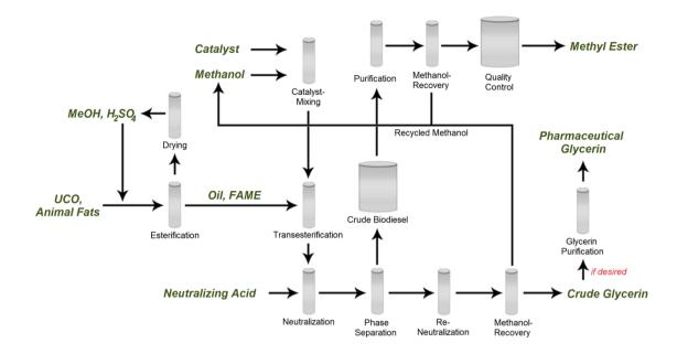
**Figure 1 Two Step Biodiesel Production Process**
