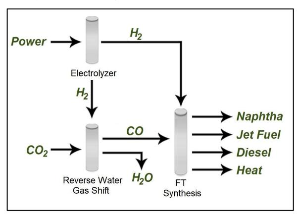
Figure 1: Power to Jet Process Flow
