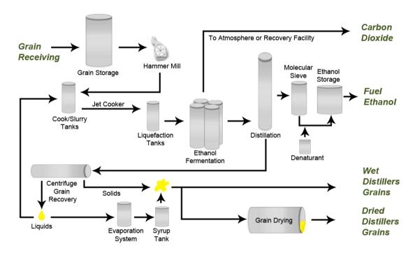
**Figure 1 1st Generation Ethanol Production Process**
