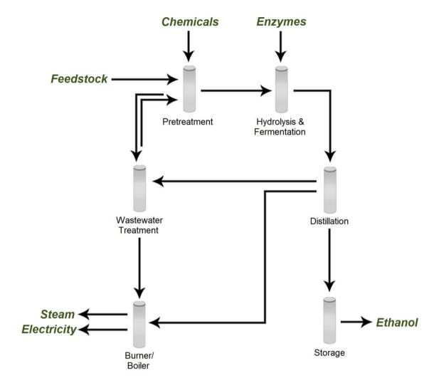
**Figure 1 Cellulosic Ethanol Process**
