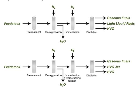
Figure 1 HVO Diesel vs Jet Process
