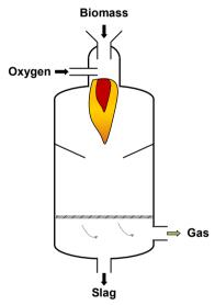
Principle of the entrained flow gasifier.
