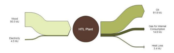
Figure 2 Hydrothermal Liquefaction Energy Balance
