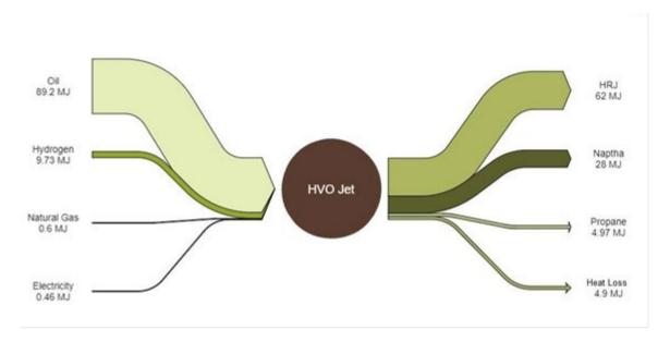
Figure 4 Alternative HVO Jet Energy Balance
