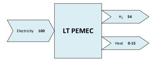
Figure 2: Example of Energy balance for LT PEMEC (2015).
