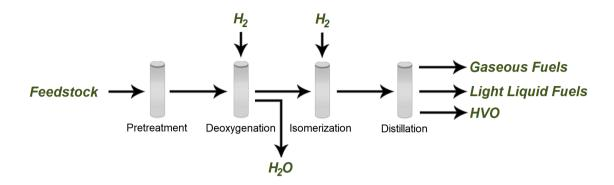
**Figure 1 HVO Production Process**
