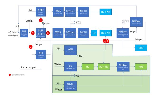
Figure 1: Different pathways for production of NH<sub>3</sub>. The light green area is the green NH<sub>3</sub> production part that is covered within this Technology Catalogue. The darker green area marks a potential future route (electrochemical). The white background shows the three conventional parts, i.e. 1a) SMR+ASU, 1b) SMR+2.REF and 2) ATR+ASU.
