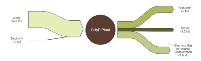
Figure 3: Catalytic Hydropyrolysis Energy Balance – Configuration 2
