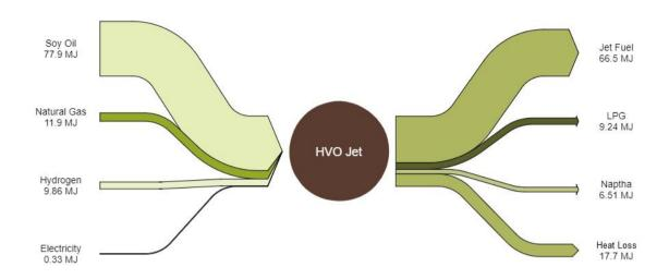
Figure 2 HVO Jet Fuel Energy Balance
