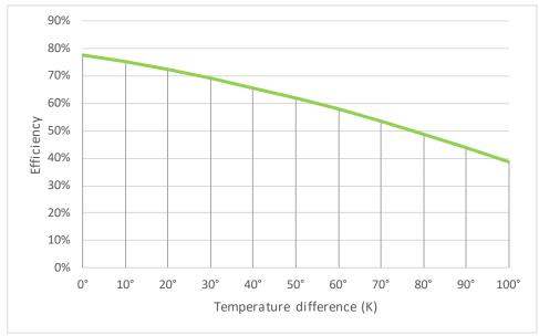
Figure 3 Efficiency as a function of temperature difference. (Based on data from [8], example with G=1.000 W/m<sup>2</sup>,  $\eta_0$ =0.777,  $a_1$ =2.41,  $a_2$ =0.015)<sup>23</sup>
