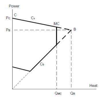
Pc: Power capacity in full condensation mode; point C. No heat production.
