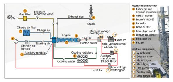
Figure 1 Large engine power plant scheme [16].
