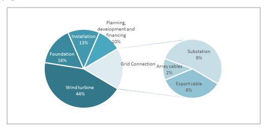
Figure 6: Breakdown of costs for offshore wind farms (Renewable Energy Technologies: Cost Analysis Series, 2012). The cost of environmental assessment is a part of the Planning & development and financing cost component
