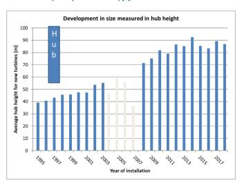
Figure 10 Average hub height for new turbines (rated power > 25 kW) [3]
