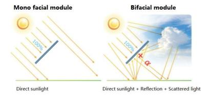
Figure 26 Bifacial module structure (Ref. 12).
