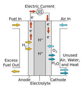
Figure 1: Diagram of a PEM-FC [2].
