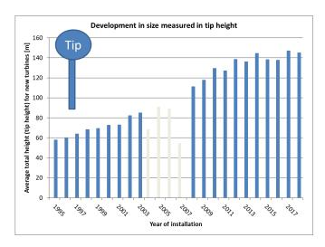
Figure 11 Average tip height for new turbines (rated power > 25 kW) [3]
