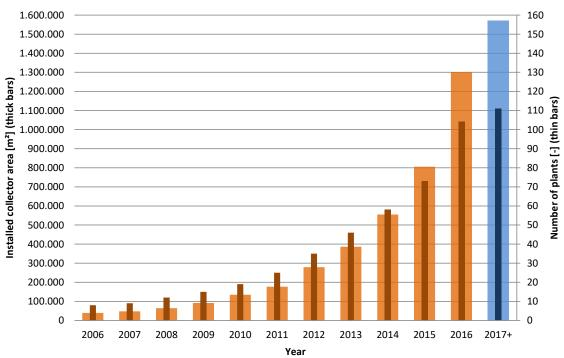
Figure 7 Solar district heating plants in Denmark in operation (until 2017) and planned. The trend is that the new plants are larger and include seasonal heat storages [5].
