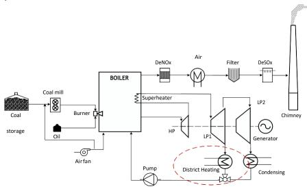
Figure 1: A schematic diagram of an extraction plant.
