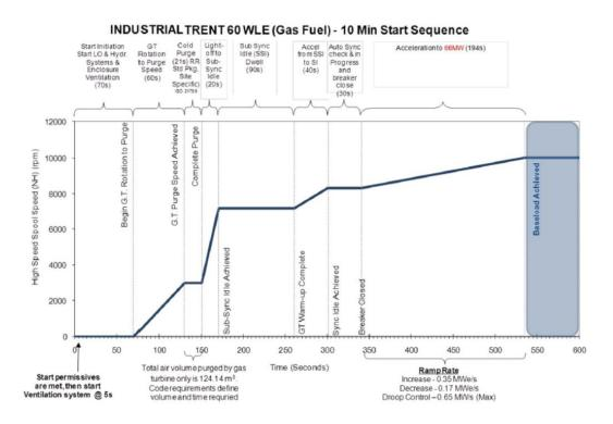
Figure 2 Start sequence and ramp rate of an aero-derivative turbine [15].
