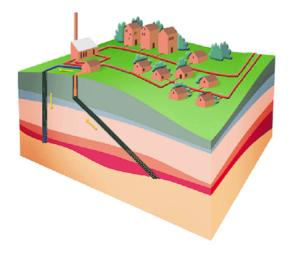
There are different concepts for extraction of the geothermal heat. In the typical doublet system, warm geothermal water is pumped to the surface from a production well, where heat is extracted via heat exchangers and possibly a heat pump and the heat depleted brine pumped back into the source reservoir via an injection well to maintain the pressure.
