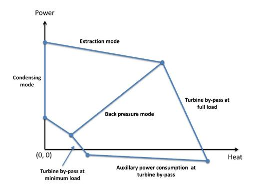
Figure 5 Generic PQ-diagram for extraction CHP
