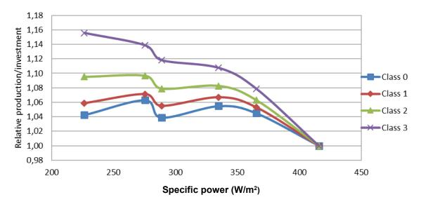
Figure 16 The production relative to the investment cost based on current available Vestas turbines for different rotor areas, generator size is 3.6 - 4 MW for all (= different specific power).
