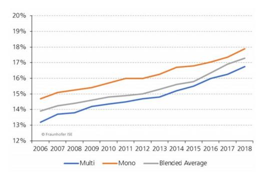
Figure 32 Efficiencies of different cell types (Ref. 9).
