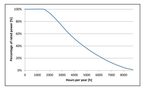
Figure 3 Example of a duration curve for a North Sea offshore wind farm [5]
