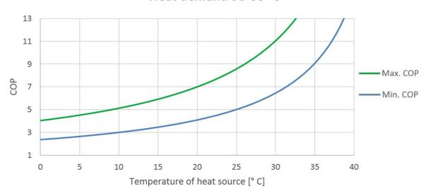
Figure 3: COP values of compression heat pump heating water from 30 to 60° C. For a heat source @ 0° C that is cooled to -5° C typical COP values will be 2.4-4.0 rising to 6.5-11 for a heat source @ 30° C that is cooled to 25° C [1].
