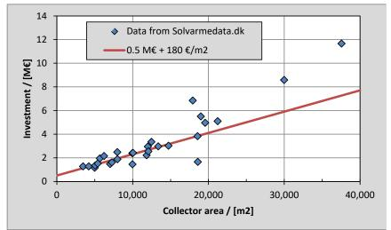
Figure 10 Solar plant investment for Danish SDH projects. The plant in the upper right corner is "Dronninglund" with 37,573 m2 which includes a seasonal heat storage – and the investment for that is 2.4 M€ (see the section below on the seasonal heat storage), bringing this plant closer to the red line [5].
