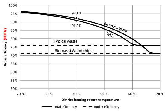
Figure 9. Total HHV-based efficiency estimate for WtE plants<sup>7</sup> and biomass plants<sup>8</sup> given varying DH return temperatures [5] – or temperature of the cold media of a heat pump.
