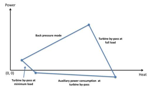
Figure 4 Generic PQ-diagram for backpressure CHP
