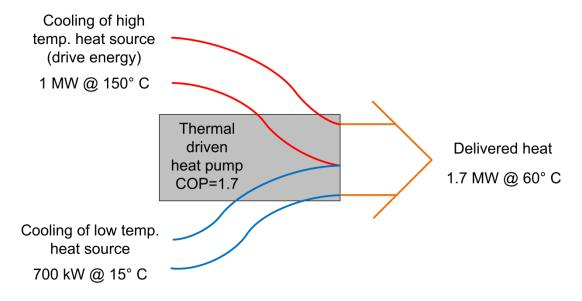
Figure 6: The high temperature drive energy of 1 MW enables the heat pump to utilize 700 kW from a low temperature heat source at 15° C. Thus delivering 1.7 MW at 60° C (COP is 1.7).
