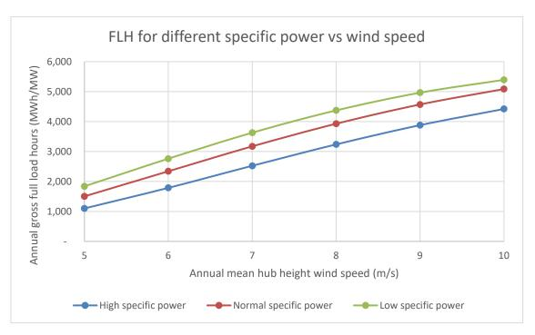
Figure 7 Annual full load hours as a function of mean wind speed at hub height. The examples in the figure are 3 MW with 90m rotor diameter, specific powers are 472 W/m2 called "high specific power" and 3.3 MW turbines with 112 m and 126 m rotor diameters, specific powers are 335 W/m² called "medium specific power" and 265 W/m² called "low specific power".
