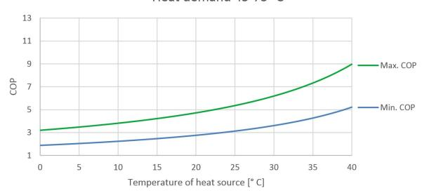
Figure 4: COP values of compression heat pump heating water from 45 to 75° C. For a heat source @ 0° C that is cooled to -5° C, typical COP values will be 2.0-3.1 rising to 5.0-9.0 for a heat source @ 40° C that is cooled to 35° C [1].
