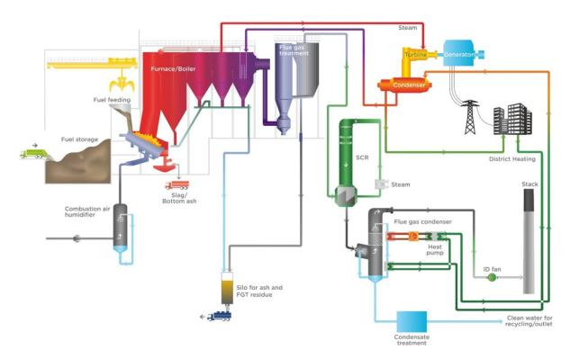
Figure 1 Main systems of a CHP (or Heat only) facility, example WtE CHP facility
