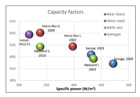
Figure 5: Capacity Factor shown as function of the Specific Power (W/m²) for Danish Offshore wind turbine projects. The 3 most left are the latest projects.
