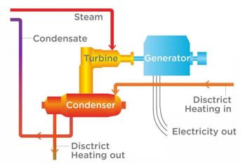
Figure 3 Turbine/generator system of backpressure CHP
