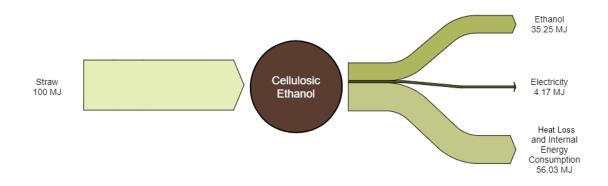
Figure 2 Cellulosic Ethanol Energy Balance
