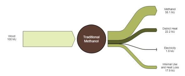
Figure 3 GreenSynFuels Traditional Methanol Plant
