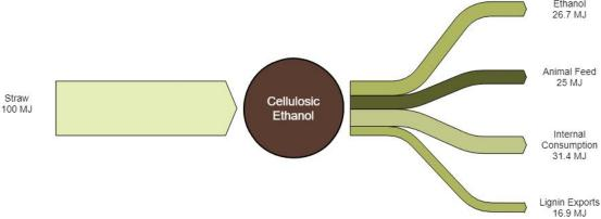
Figure 4 Inbicon Cellulosic Ethanol Energy Balance
