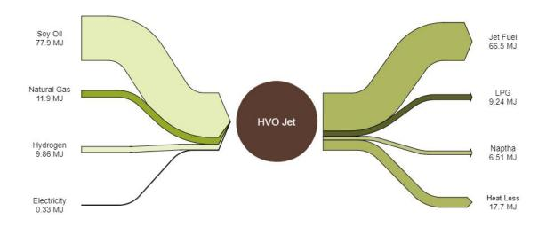
Figure 2 HVO Jet Fuel Energy Balance
