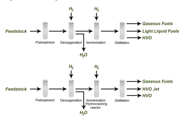
Figure 1 HVO Diesel vs Jet Process
