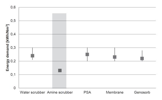
Figure 3: Electricity consumption (kWh/Nm³ raw biogas, indicated as box and line) for the upgrading technologies, water scrubber, chemical/amine scrubber, PSA, membrane separation and organic physical scrubbing (Genosorb). Heat consumption shown as column. Source: SGC (2013).
