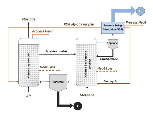
Figure 5. Fluidized Bed Catalytic-assisted Decomposition Diagram.
