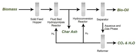
Figure 1: Catalytic Hydropyrolysis Process Flow
