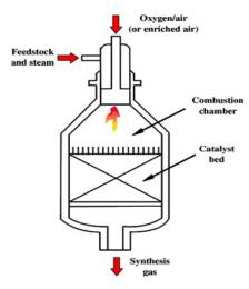
Figure 5: Autothermal reformer (ATR)
