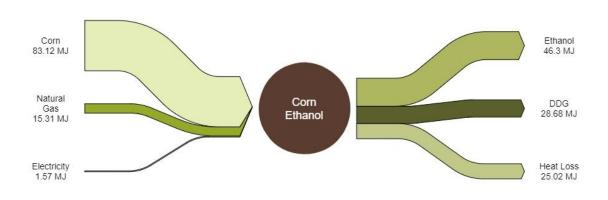
Figure 2 1st Generation Ethanol Energy Balance
