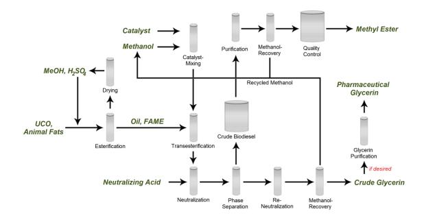
**Figure 1 Two Step Biodiesel Production Process**
