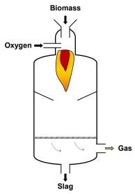
Principle of the entrained flow gasifier.
