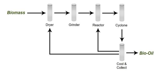
Figure 1 Fast Pyrolysis Process Flow
