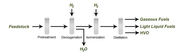
**Figure 1 HVO Production Process**
