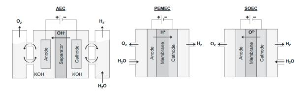
Figure 1: Operating principle of AEC, PEMEC and SOEC [1].
