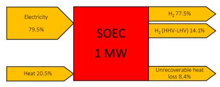
Figure 4: Energy balance (2020) for a 1 MW solid oxide electrolysis cell compared on LHV basis.
