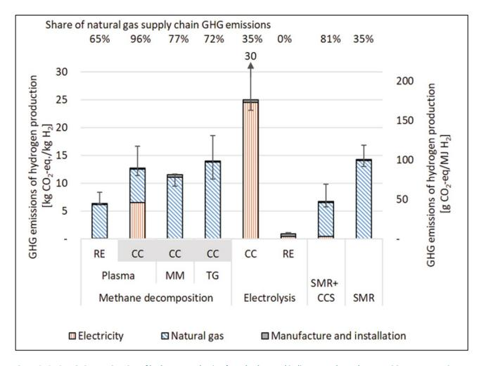
Figure 8. GHG emissions estimation of hydrogen production (grey background indicates methane decomposition systems using natural gas as basis for process energy; electricity from combined cycle power plants (CC) or renewable energy (RE); methane decomposition in molten metal (MM) and thermal gas (TG, i.e. MBR) system; steam methane reforming (SMR) without or with CO<sub>2</sub> capture and storage (+CCS)), (Ref. [11])
