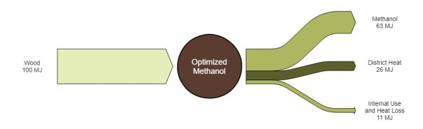
**Figure 4 Optimized Biomass to Methanol Plant**
