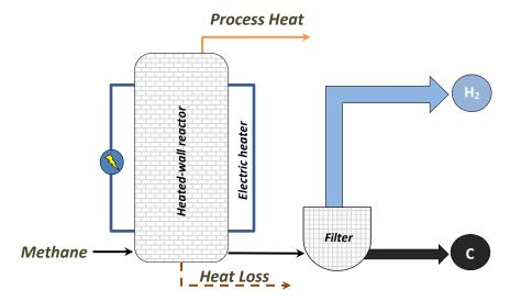
Figure 1. Thermal-assisted (heated-wall) Decomposition Diagram.
