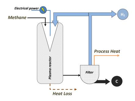
Figure 4. Plasma-assisted Decomposition Diagram.
