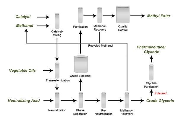
**Figure 1 Biodiesel Production Process**
