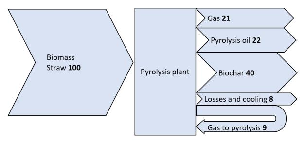
Figure 3. Example of energy balance for slow pyrolysis of straw, 10% incoming moisture content. All inputs sum to 100 units. Note, the balance shows the core process only. Assumed pyrolysis temperature is 550-600°C. The gas to pyrolysis stream can be seen as an internal stream in the pyrolysis plant, as a fraction of the output gas is recirculated into the pyrolysis process.
