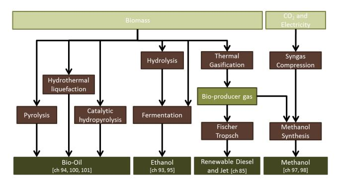
Figure 4 Pathways for biomass to liquid fuels and CO<sub>2</sub> + electricity to liquid fuels
