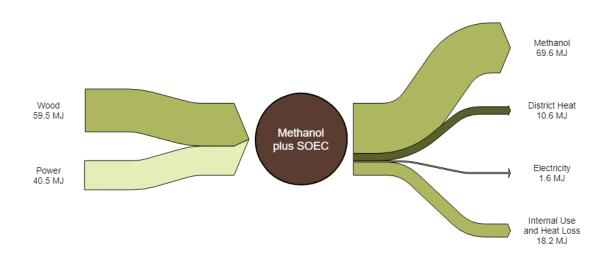
Figure 5 Hybrid Biomass to Methanol Plant
