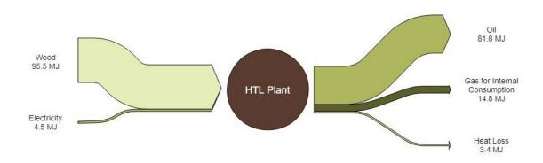
Figure 2 Hydrothermal Liquefaction Energy Balance
