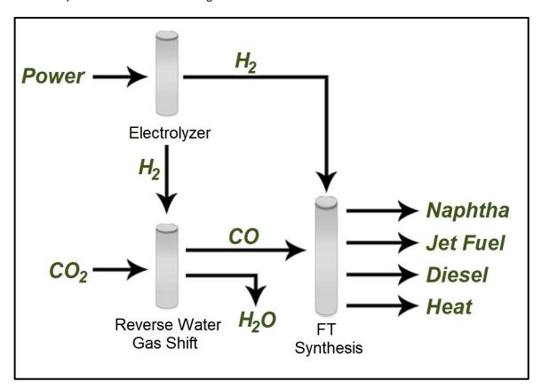
Figure 1: Power to Jet Process Flow
