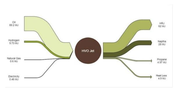
Figure 4 Alternative HVO Jet Energy Balance
