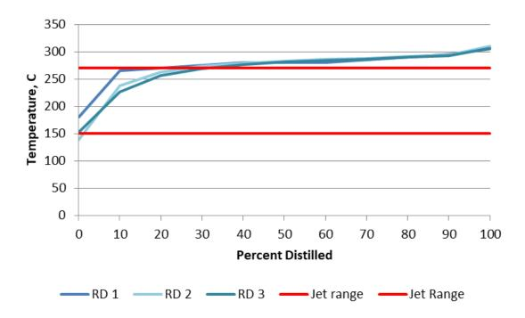
**Figure 5 Renewable Diesel Distillation Curves**
