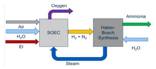
Figure 11: SOC4NH3 project combining electrolysis unit and ASU (El = power)[ref 15]
