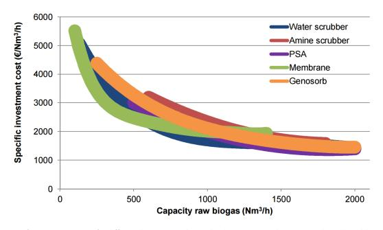
Figure 1: Specific investment costs for different biogas upgrading technologies. Genosorb is organic physical scrubbing. Source: SGC (2013).
