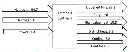
Figure 12: Overall energy balance of the ammonia synthesis. The electrolysis unit is covered in [4] and power required for the ASU is listed in Table 1.
