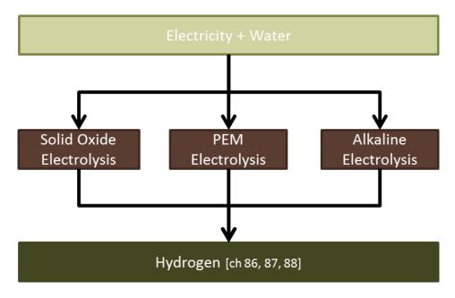
Figure 2 Pathways for hydrogen production from electricity (PEM: Polymer electrolyte membrane or Proton exchange membrane)
