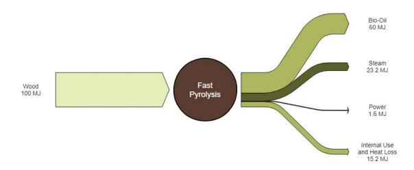
Figure 2 Fast Pyrolysis Oil Energy Balance
