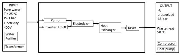
Figure 5: A sketch of an electrolysis system for AEC and PEM.
