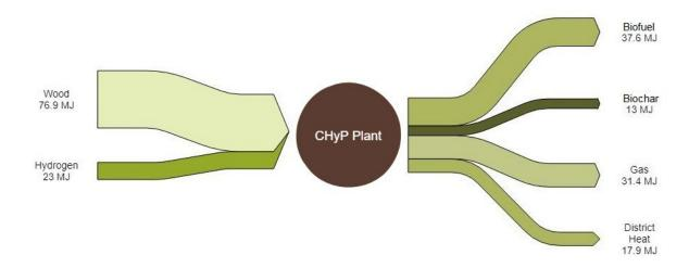
Figure 2: Catalytic Hydropyrolysis Energy Balance – Configuration 1
