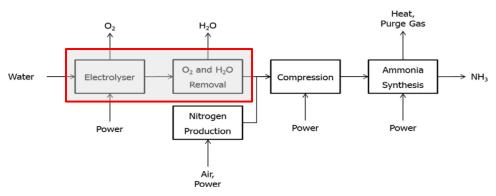
Figure 3: Green ammonia plant. Any impurities of O<sub>2</sub> in the H<sub>2</sub> product is removed by reacting it with H<sub>2</sub> over a DeOX (deoxygenation unit).
