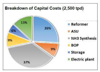
Figure 15. Cost split on main systems in a conventional NH<sub>3</sub> plant from Linde [10]. Reformer, electric plant (power plant) and some balance of plants (BOP) will disappear for a green NH<sub>3</sub> plant. Cost of green NH<sub>3</sub> plant (excl. electrolysis unit and ASU) is therefore taken as 54% of conventional plant, based on all obtained data.
