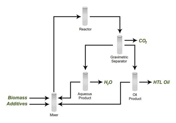
Figure 1 Hydrothermal Liquefaction Process Flow
