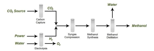
**Figure 1 Methanol to Power Process**
