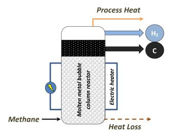
Figure 2. Thermal-assisted (Molten Metal) Decomposition Diagram.
