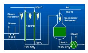
Figure 4: Primary and secondary reformer arrangement
