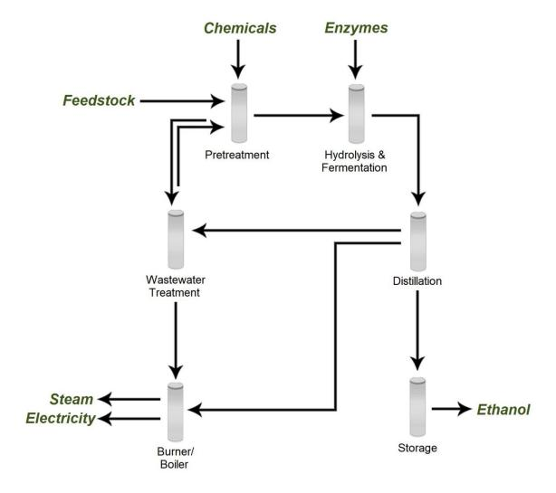
Figure 1 Cellulosic Ethanol Process
