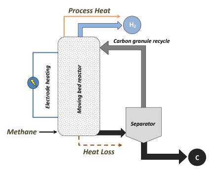
Figure 3. Thermal-assisted (moving-bed reactor) Decomposition Diagram.
