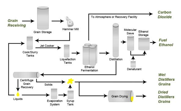
**Figure 1 1st Generation Ethanol Production Process**
