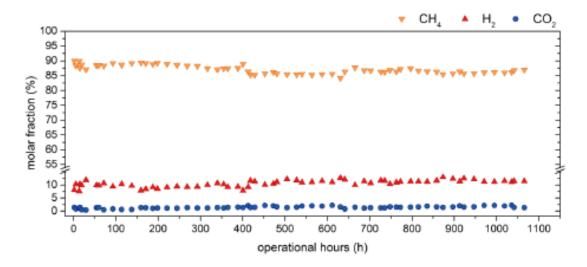
Figure 5 Gas Composition Prior to Final Clean-up
