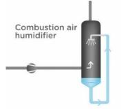
Figure 8 Combustion air humidifier, where water heated by a low-temperature source is evaporated into the combustion air flow.
