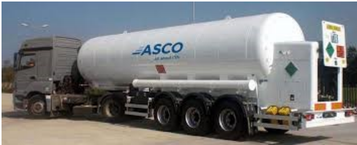
Figure 50. CO 2 semi-trailer from ASCO. Source; www.ascoCO2.com
