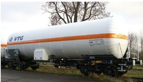
Figure 51. Railroad car for liquid CO 2 transport. Source: www.VTG.com
