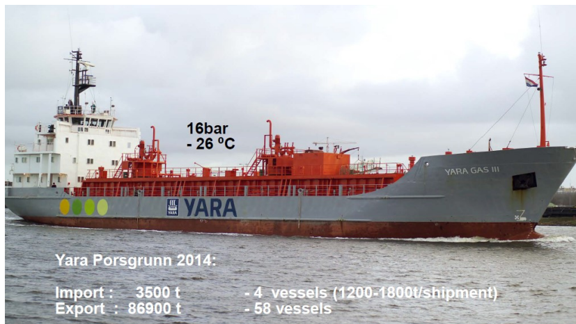
Figure 49. M/T Yara Gas III liquid CO 2 carrier. [7]
