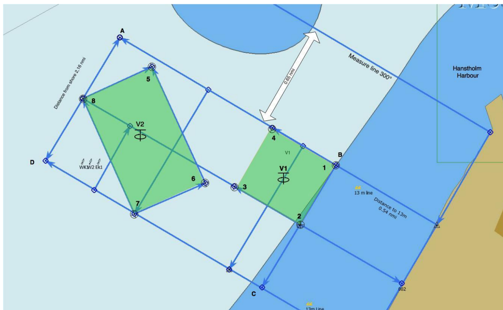
Figure 1: Sea chart showing the desired location of the test anchors at „V6“.
