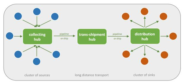
Figure 3: Schematic illustration of a CCS infrastructure. (Source: BGR).
