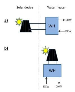
Figure 1 Examples of a) package of water heater and solar device and b) a solar water heater
