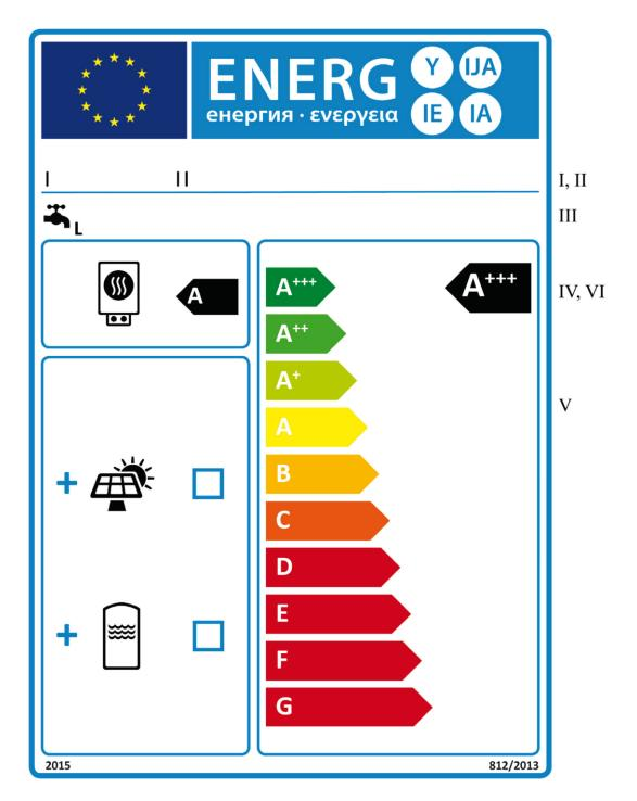
Figure 3 Water heater package label
