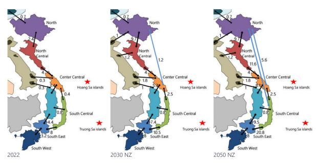
Figure 5.6 Installed transmission lines in GW in 2022, 2030 and 2050 in the Net-Zero scenario (black lines indicate HVAC connections, and blue lines indicate HVDC connections).
