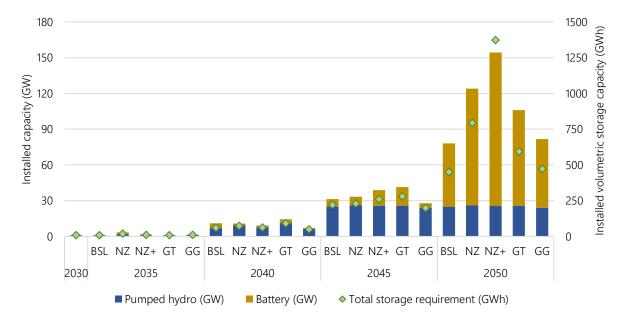
Figure 5.9 Battery and pumped storage capacities (GW) and total volumetric storage capacity (GWh).
