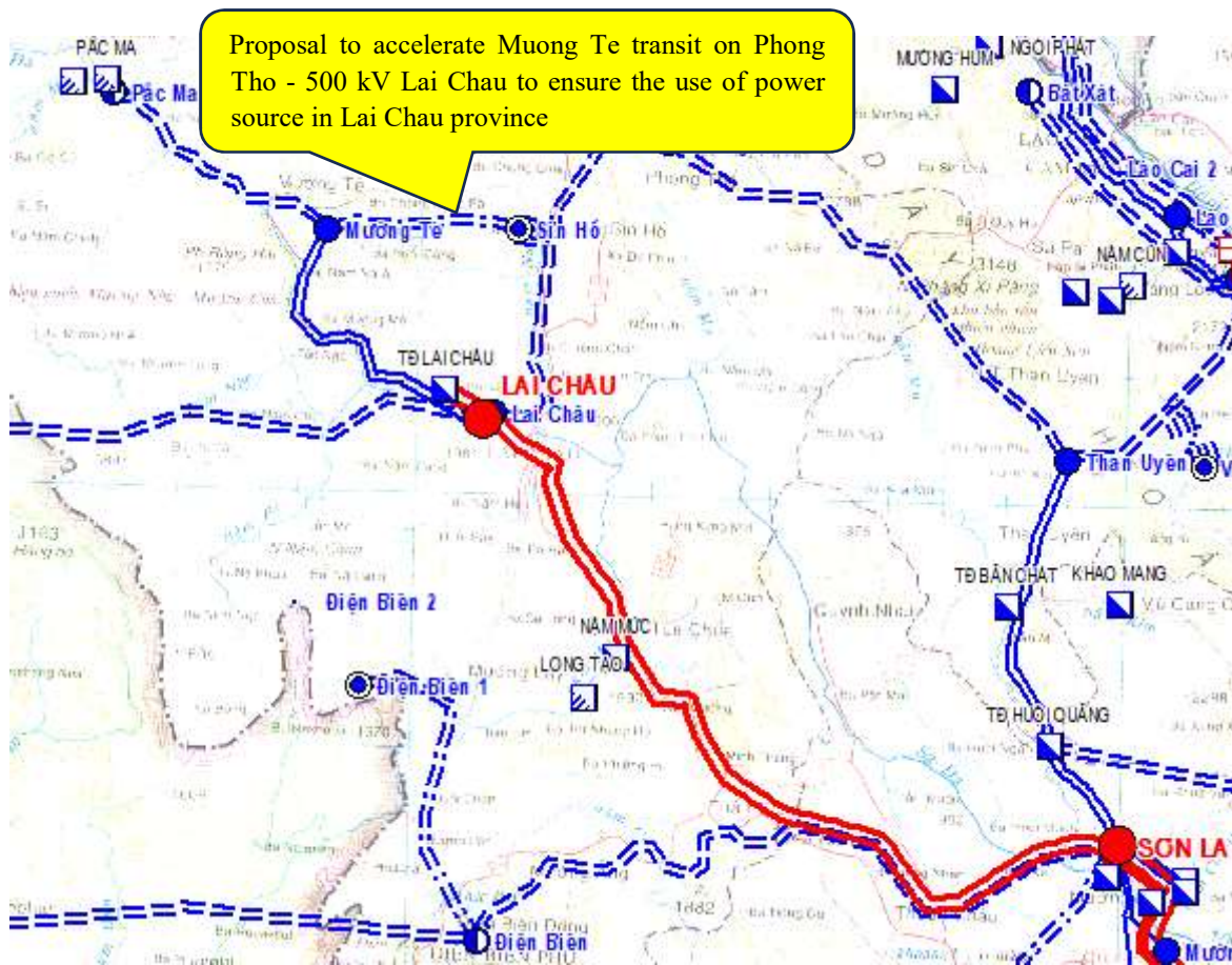
Figure 15 Transmission grid map in North West.
