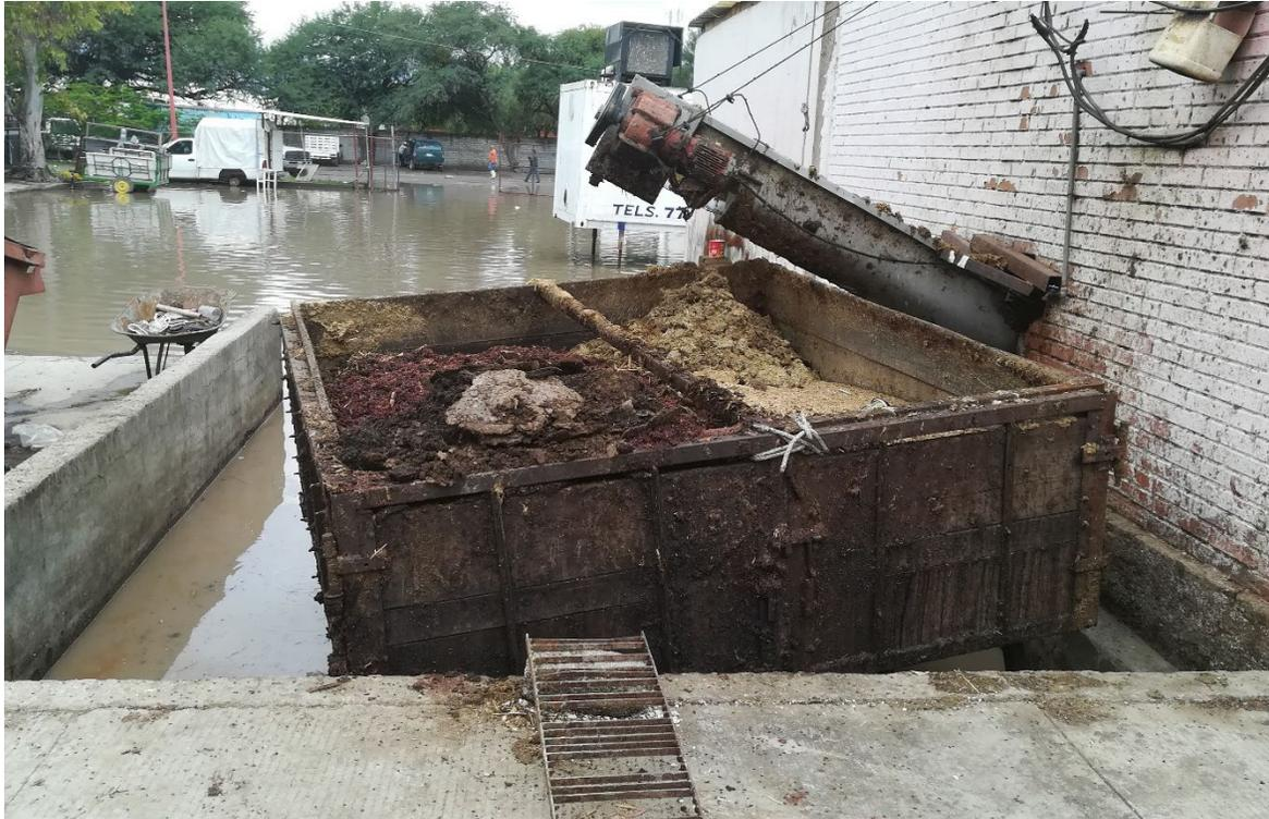
**Figure 26. Conveyor screw to the truck (for subsequently composting)**
