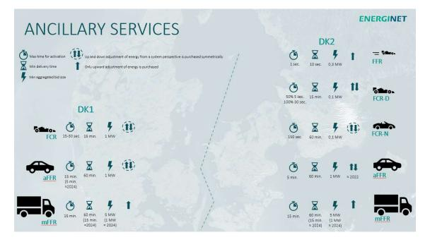
Figure 3. Technical specifications for ancillary services in Denmark
