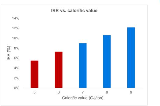
Figure 10 – Sensitivity assessment of IRR compared to the calorific value of waste
