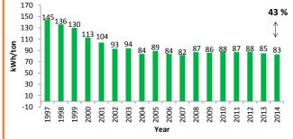
Figure 2. Development in electricity consumption per ton malt.
