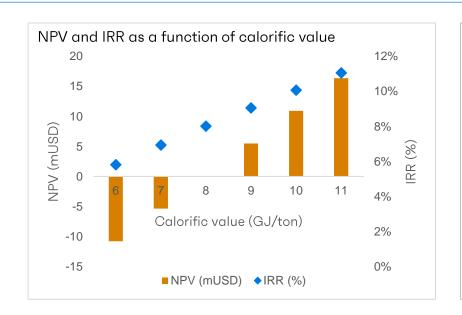
Calorific value, also called *heating value*, has a significant impact on power production (yield).
