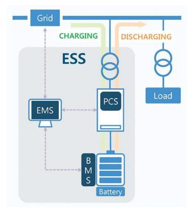
Figure 2 Illustration of the components of a BESS [2]
