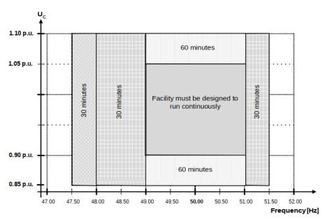
Figure 5 Operating time requirement across voltage ranges for a BESS [4]
