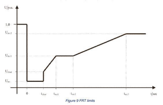
Fault-ride-through profile of a power-generating module
