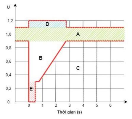
Figure 1-1. Illustration of the fault-ride-through of a BESS
