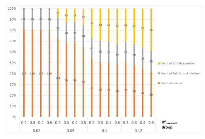
Figure 9 Simulation results for different frquency thresholds between 50.2 and 50.5 Hz and LFSM-O droop settings between 2% and 12% [8]
