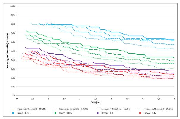
Figure 8 Percentage of stable scenarios depending on respond time and LFSM-O parameters
