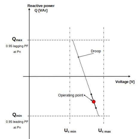
Figure 1-3. Illustration of the reactive-voltage droop characteristic of a BESS [9]
