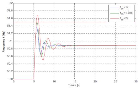
Figure 8 Time domain response for one exemplary scenario with different response times. [8]
