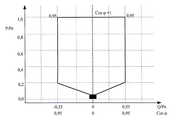
Figure 1-2. Illustration of the reactive power regulation characteristic of a BESS
