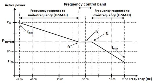
Figure 4 Active power control characteristics of a BESS in the frequency range [4]
