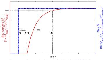
Figure 7 Evaluating the required time behavior of LFSM-O [8].
