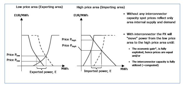
Figure 6: Principle of joint scheduling of generation and transmission for two interconnected bidding areas
