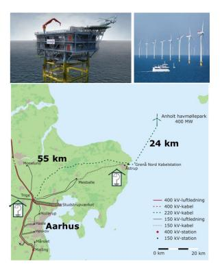
Figure 56: Connection of Anholt 400 MW offshore wind farm
