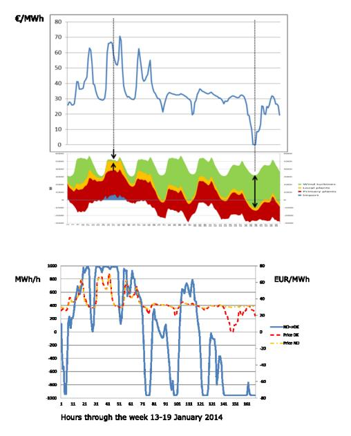
Figure 54: Price volatility due to variations in wind power generation. Interconnector capacity to e.g. Norway (capacity ~1,000 MW in 2014) is intensively used in the market balancing process. (Import to Denmark has positive value).
