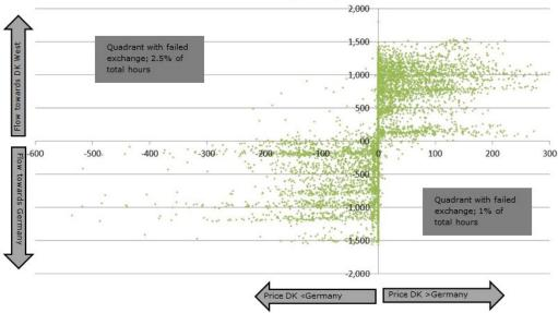
Exchange (MWh/h) between DK West and Germany as a function of price difference DKK/MWh (2013)
