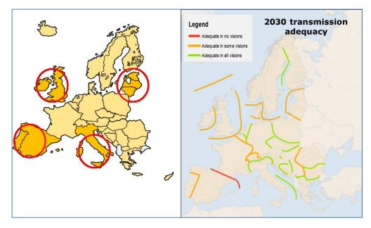
Figure 41: Right: Illustration of transmission adequacy; left: four "electric peninsulas"
